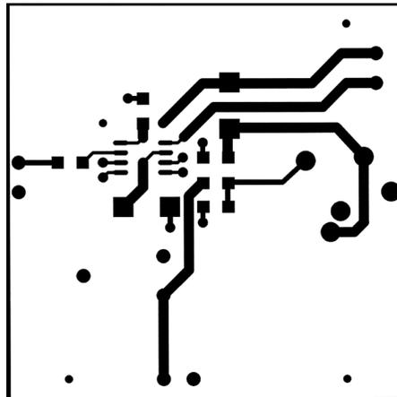
Figure 29. Recommended SOIC PC Board Layout:
