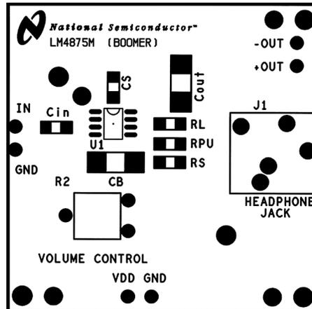
Figure 28. Recommended SOIC PC Board Layout:
