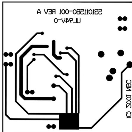
Figure 30. Recommended SOIC PC Board Layout:
