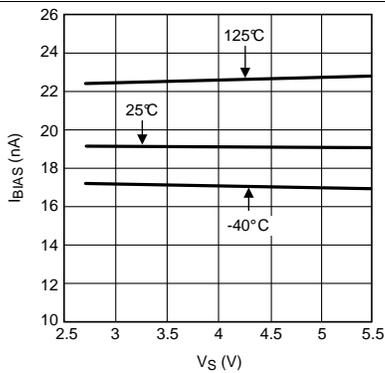
**Figure 21.  $I_{BIAS}$  vs Supply Voltage**
