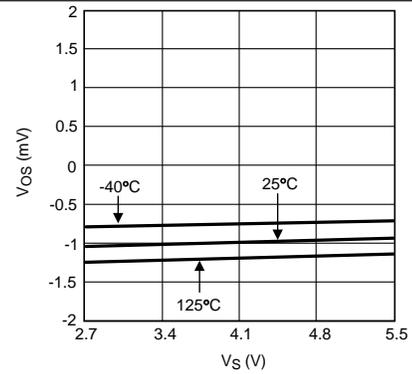
Figure 18. Vos vs Supply Voltage
