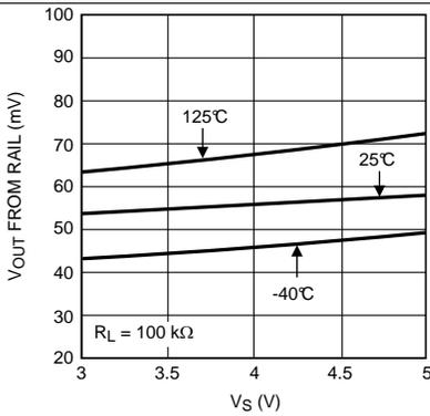
**Figure 23. Negative Output Swing vs Supply Voltage**
