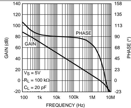
Figure 4. Open-Loop Gain and Phase With Resistive Load
