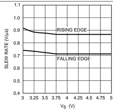
Figure 6. Slew Rate vs Supply voltage
