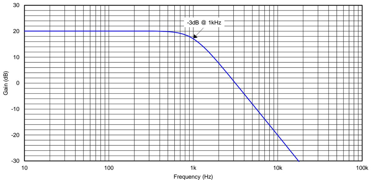
**Figure 31. 1KHz, 2-Pole Sallen-Key Low Pass Filter Results**
