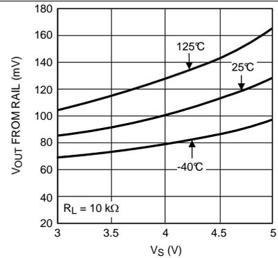
**Figure 22. Positive Output Swing vs Supply Voltage**
