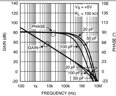
Figure 1. Open-Loop Gain and Phase With Capacitive Load
