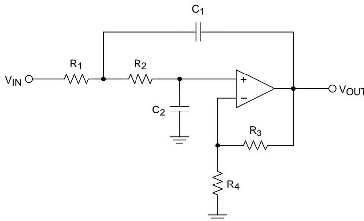
**Figure 29. Two Pole Sallen-Key Low Pass Filter**
