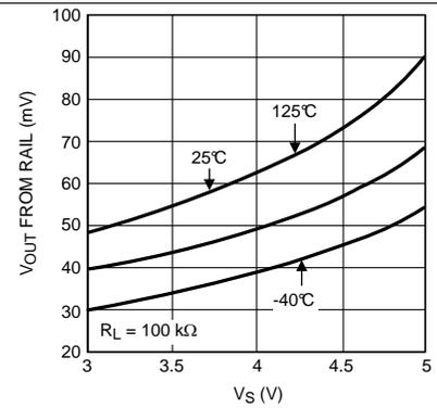
**Figure 24. Positive Output Swing vs Supply Voltage**
