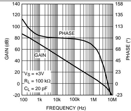
Figure 2. Open-Loop Gain and Phase With Resistive Load
