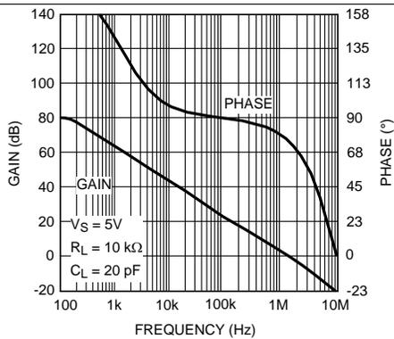
Figure 5. Open-Loop Gain and Phase With Resistive Load
