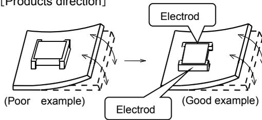
The electrode part of the products should be located like the picture to the mechanical stress.
