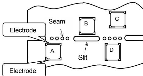
\*1 A > D is valid when stress is added vertically to the perforation as with Hand Separation. If a Cutting Disc is used, stress will be diagonal to the PCB, therefore A > D is invalid.
