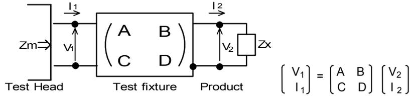
(2) The impedance of chip coil Zx and measured value Zm can be described by input/output current/voltage.
