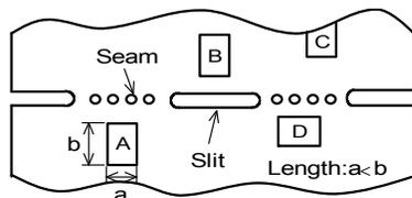
\*1  $A > D$  is valid when stress is added vertically to the perforation as with Hand Separation.
