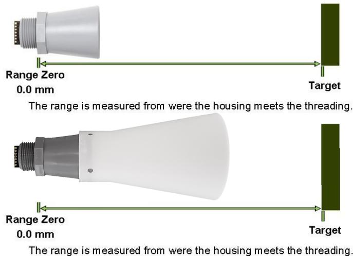
In general, the HRXL-MaxSonar-WR will report the range to the leading edge of the closest detectable object. Target detection has been characterized in the sensor beam patterns.
