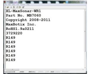
The serial data format is 9600 baud, 8 data bits, no parity, with one stop bit (9600-8-N-1). On power up the sensor will send serial data about the sensor. [View an example here.](#)
