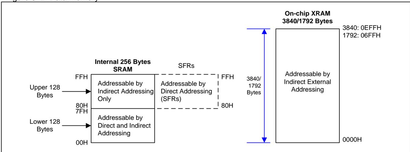
Figure 6–3. Lower 128 Bytes of Internal RAM
