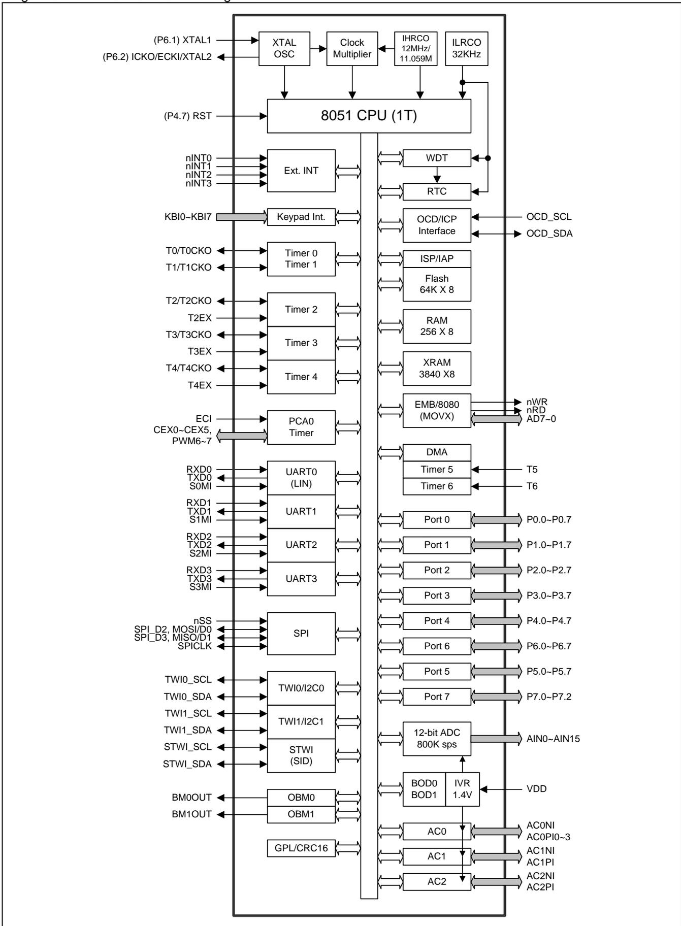
Figure 2–2. MG82G6D32 Block Diagram
