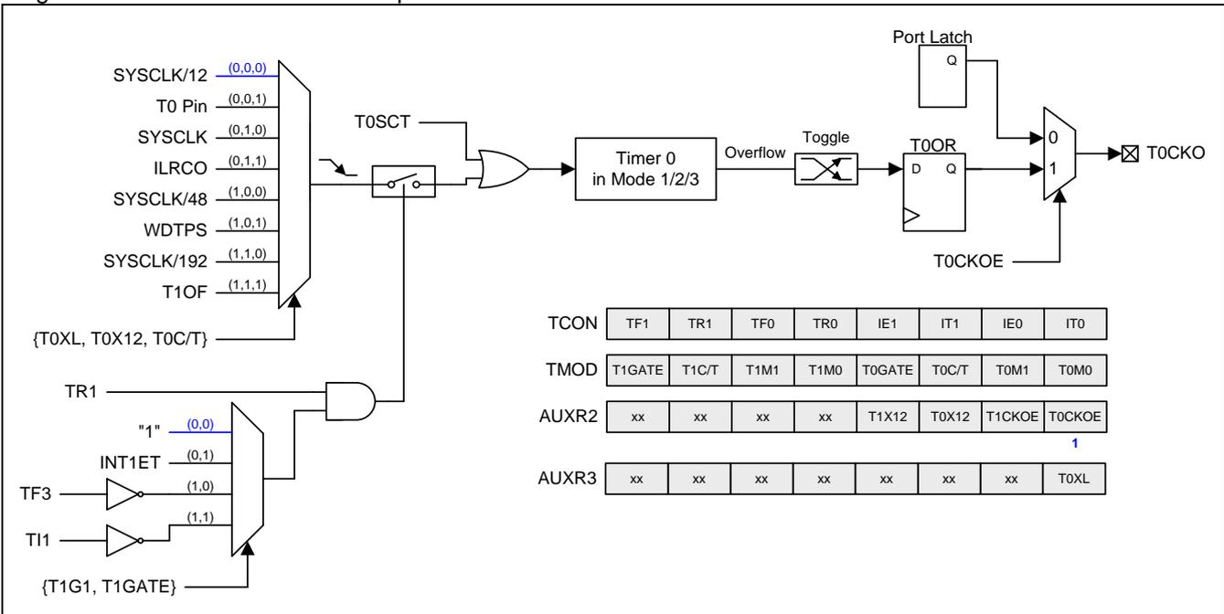
Figure 16–11. Timer 0 Clock Output Control
