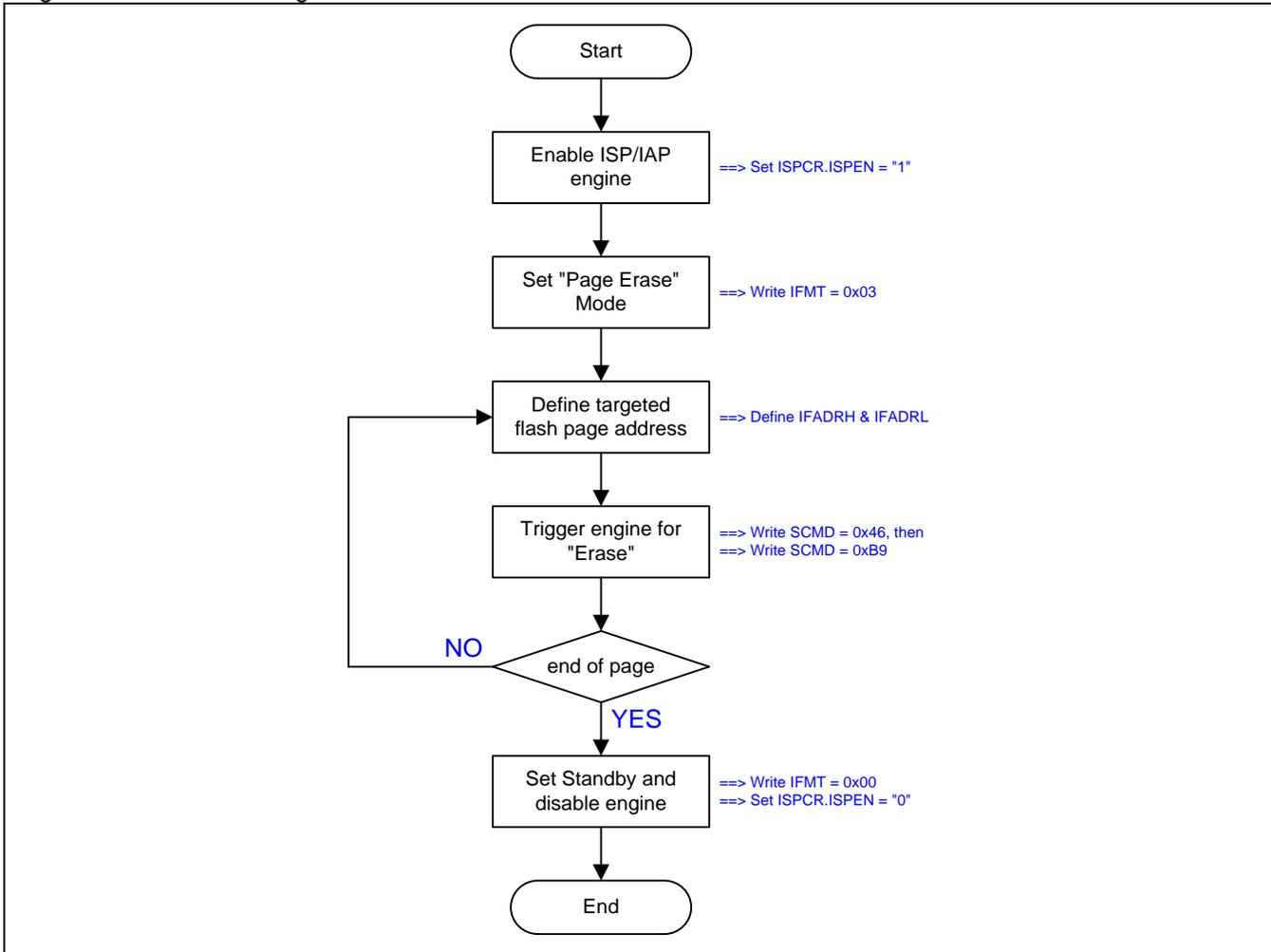
[Figure 32–4](#) shows the demo code of the ISP/IAP page erase operation.
