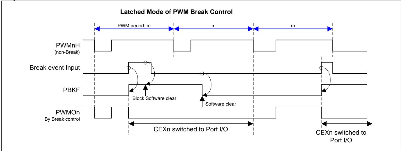
Figure 17–18. Cycle-by-Cycle Mode Waveform of PWM Break control
