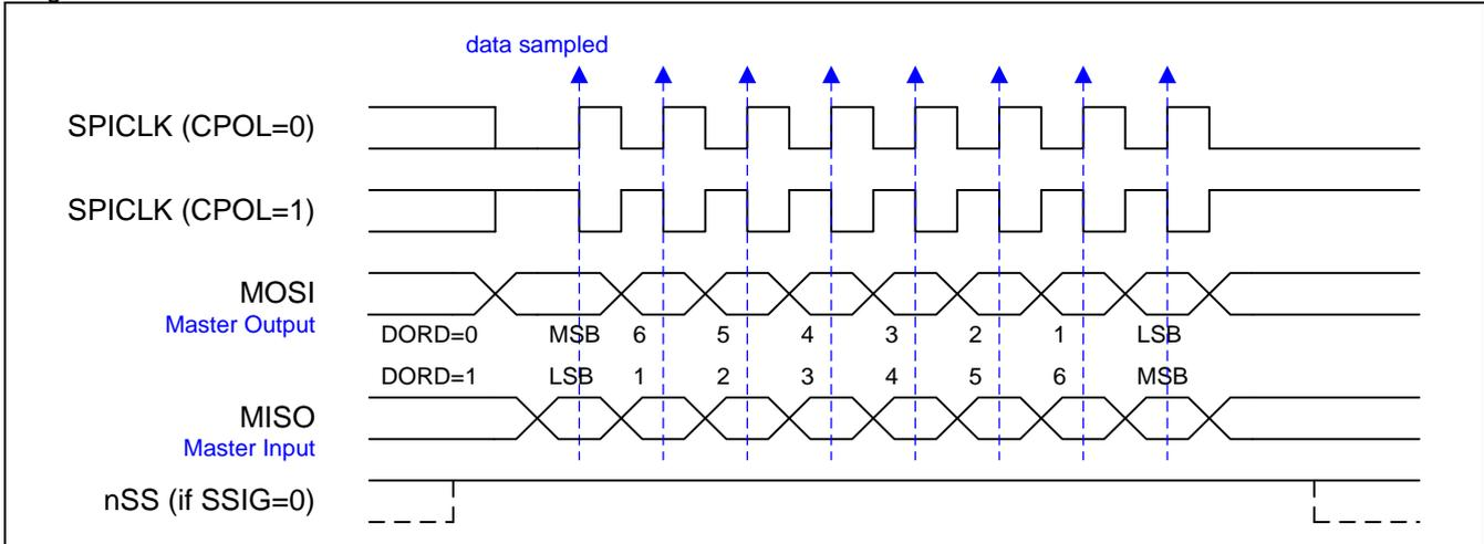
Figure 22–8. SPI Master Transfer Format with CPHA=1
