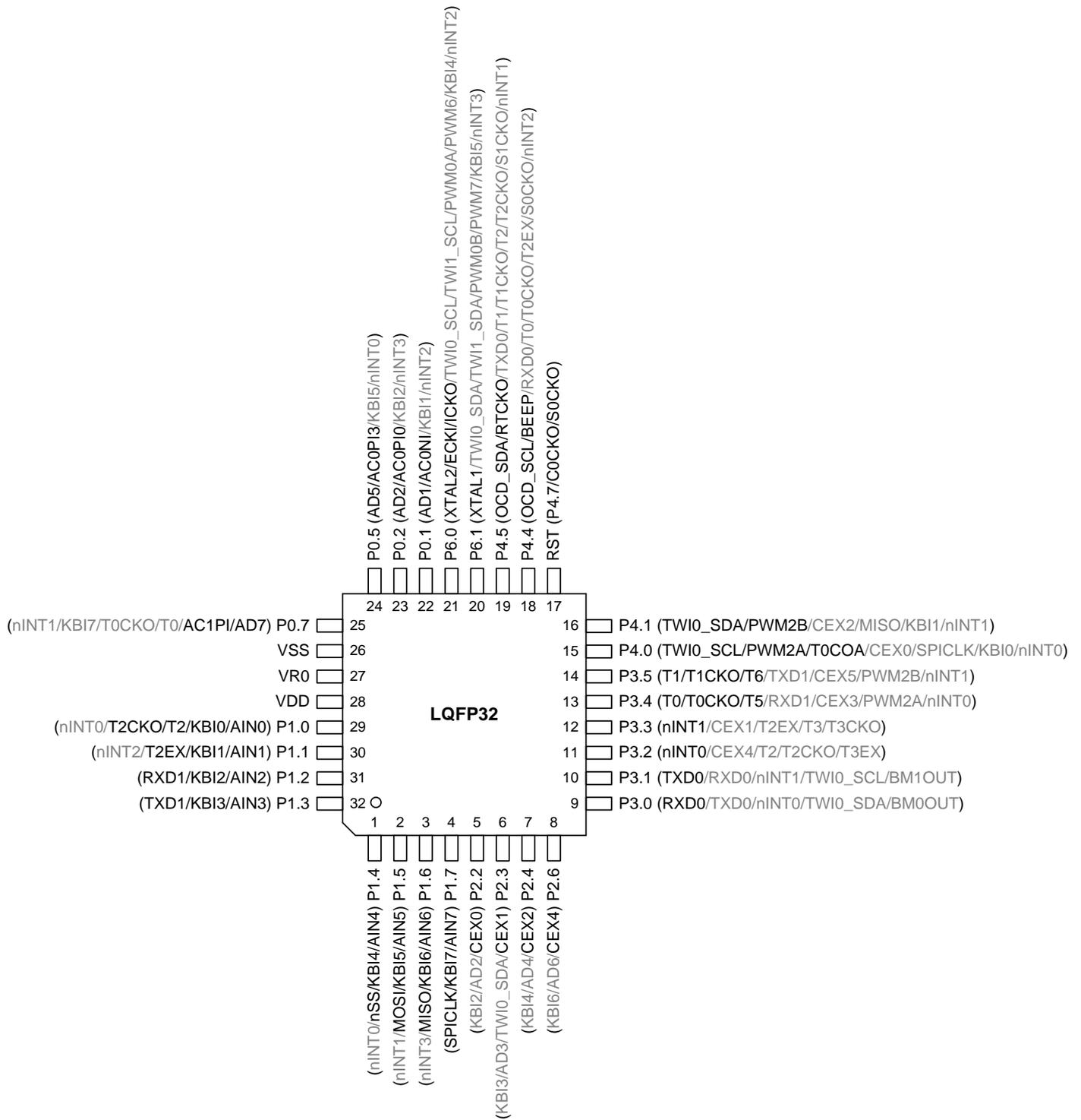
Figure 4–6. **MG82F6D32AZ32** QFN32 Top View
