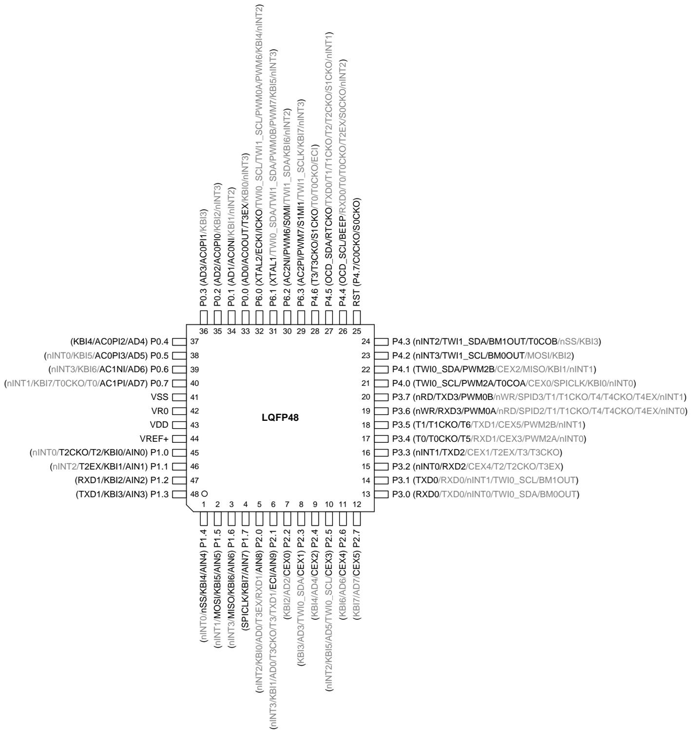
Figure 4–3. MG82F6D32AD48 LQFP48 Top View
