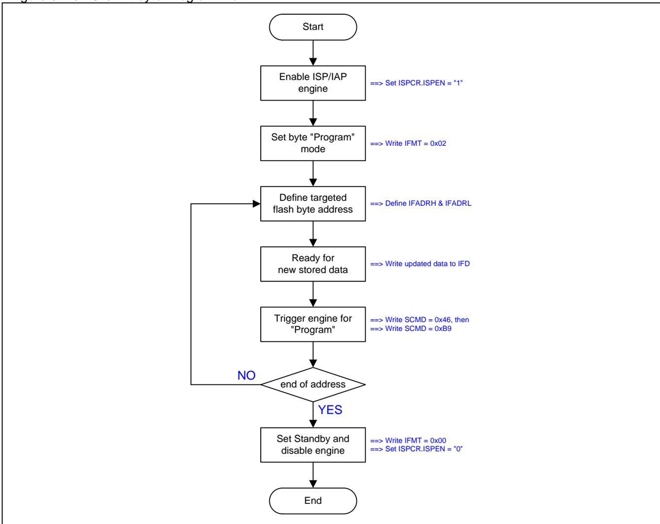
Figure 32–6 shows the demo code of the ISP/IAP byte program operation.
