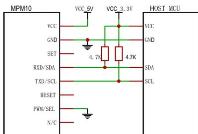
Electrical connection of IIC interface
