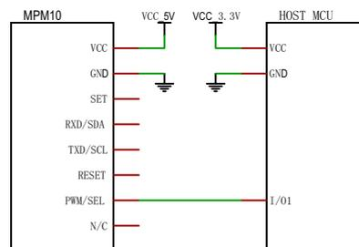
Electrical connection of PWM output
