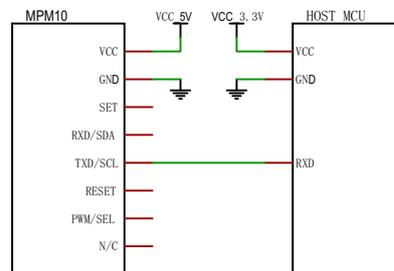
The simplest circuit connection of UART
