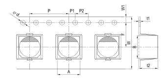
Taping Specification for SMD Type of OP-CAP
