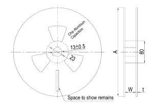
Fig. 2-2 Reel Polarity
