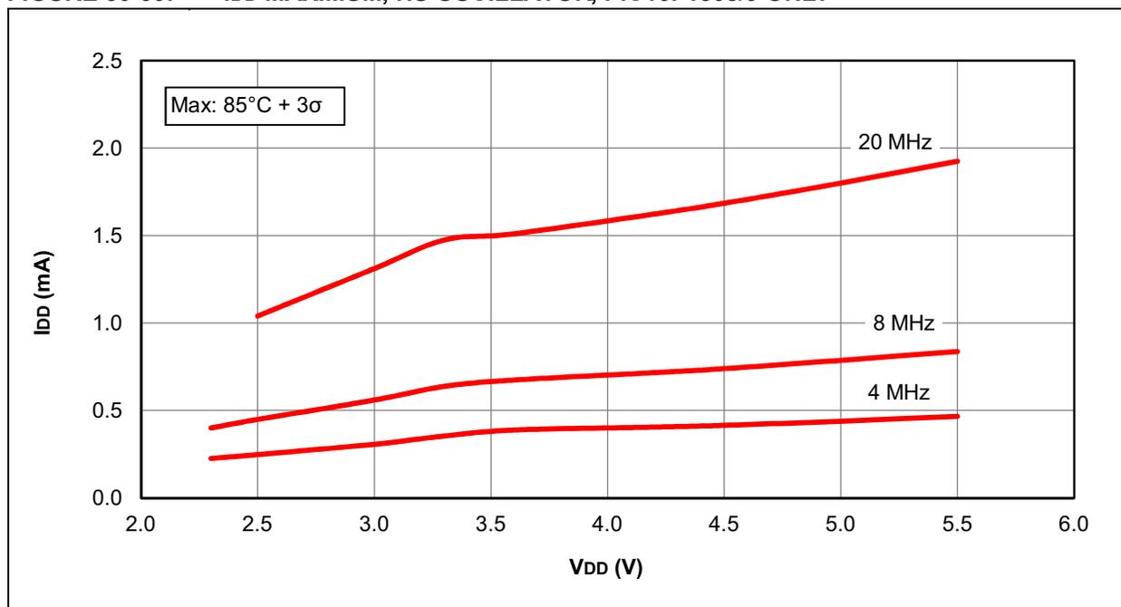
**FIGURE 30-31: I<sub>PD</sub> BASE, LOW-POWER SLEEP MODE, PIC16LF1508/9 ONLY**
