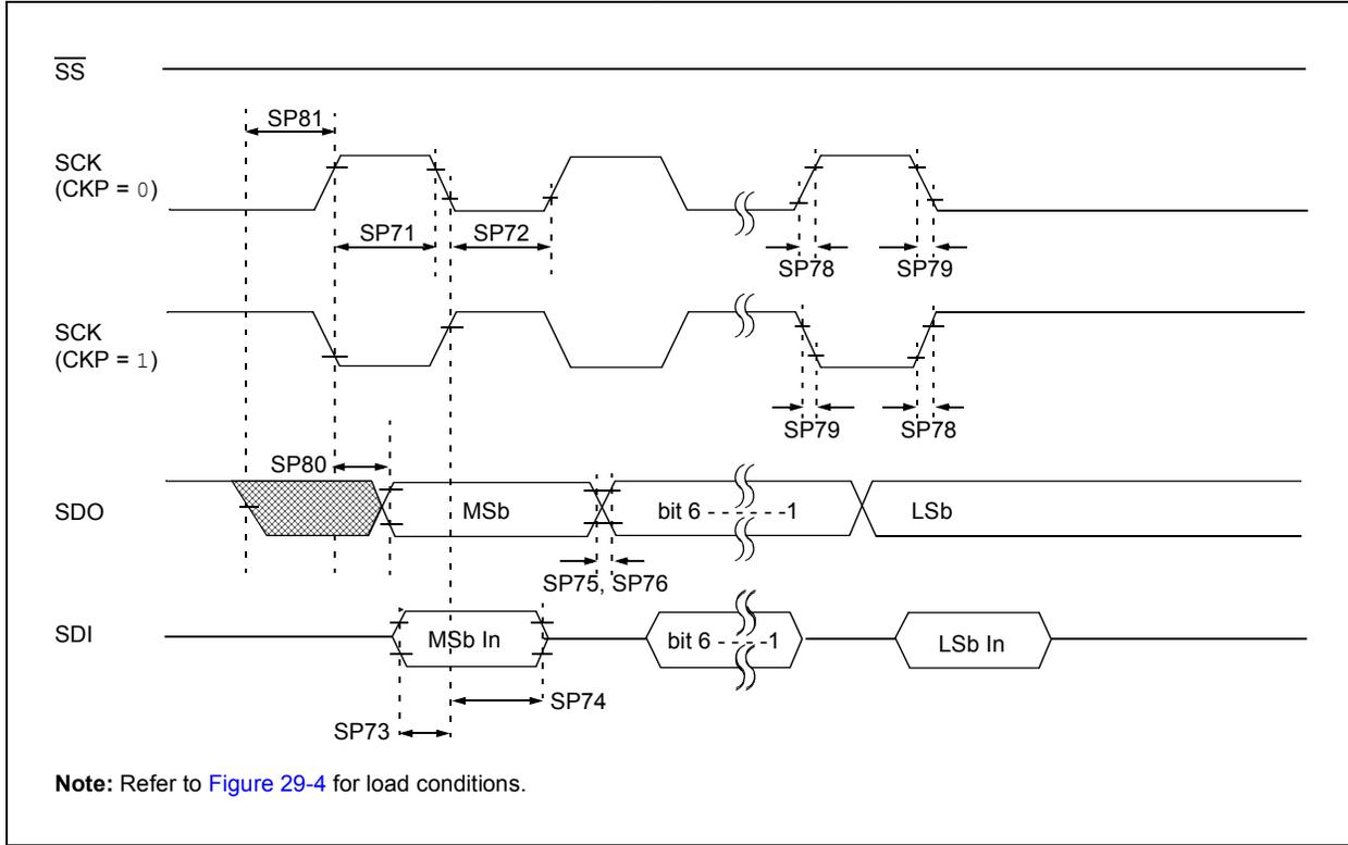
**FIGURE 29-17: SPI MASTER MODE TIMING (CKE = 1, SMP = 1)**
