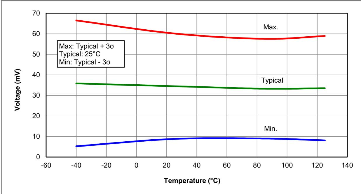
FIGURE 30-59: BROWN-OUT RESET VOLTAGE, BORV = 0
