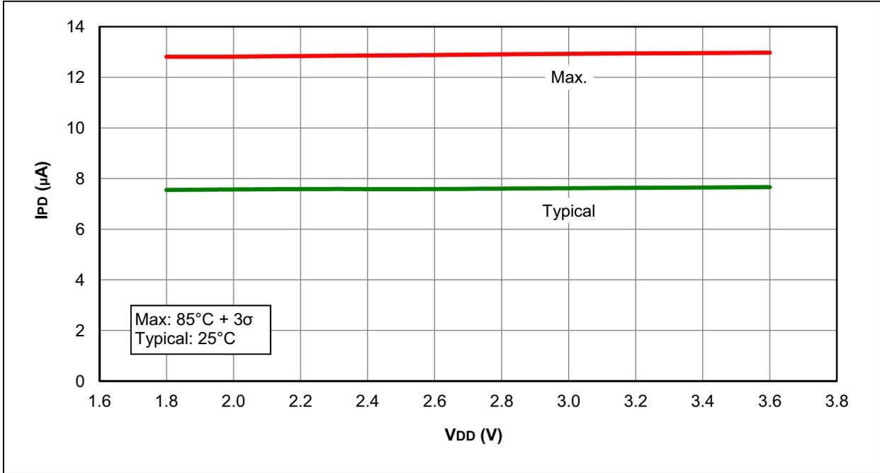
**FIGURE 30-44: I<sub>PD</sub>, COMPARATOR, LOW-POWER MODE (C<sub>x</sub>SP = 0), PIC16F1508/9 ONLY**
