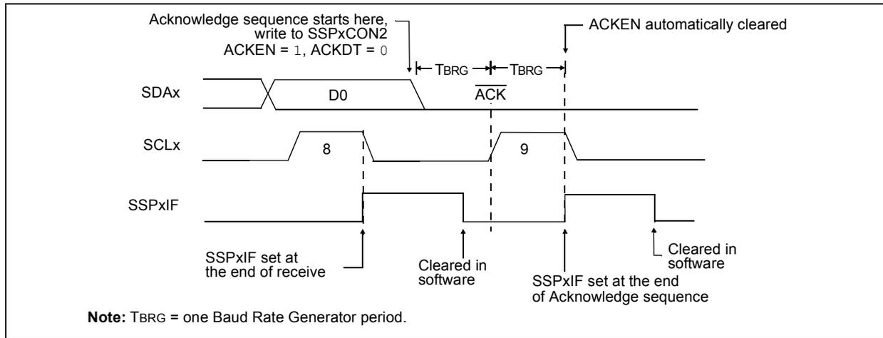
**FIGURE 21-31: STOP CONDITION RECEIVE OR TRANSMIT MODE**
