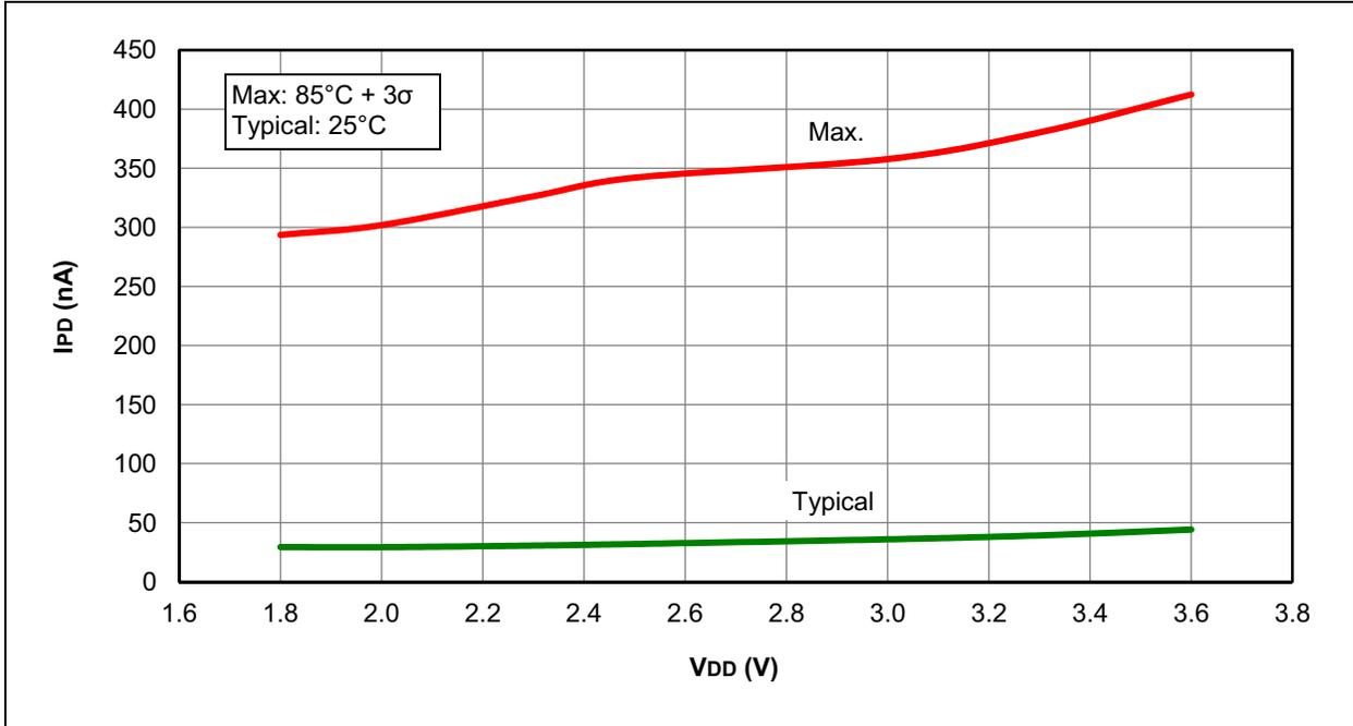
**FIGURE 30-32: I<sub>PD</sub> BASE, LOW-POWER SLEEP MODE, VREGPM = 1, PIC16F1508/9 ONLY**
