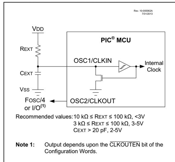
The RC oscillator frequency is a function of the supply voltage, the resistor (REXT) and capacitor (CEXT) values and the operating temperature. Other factors affecting the oscillator frequency are:
