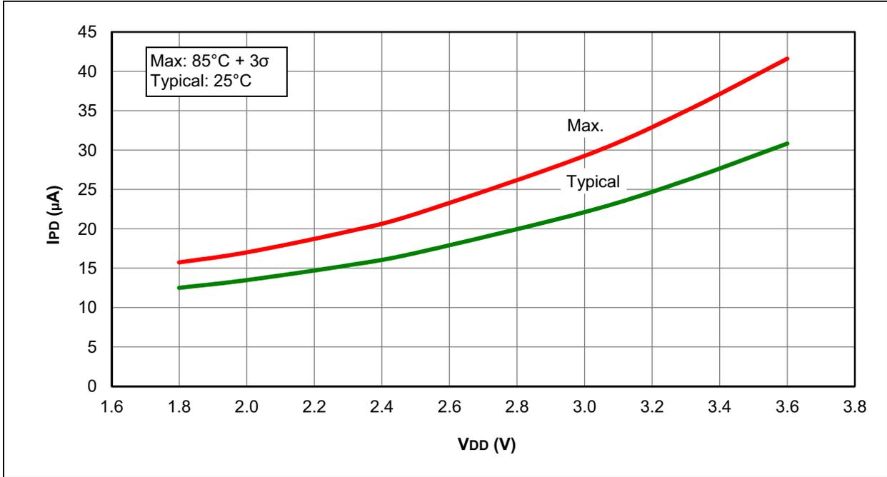
**FIGURE 30-36: I<sub>PD</sub>, FIXED VOLTAGE REFERENCE (FVR), PIC16F1508/9 ONLY**
