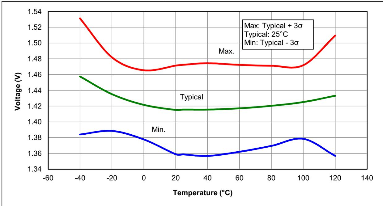
**FIGURE 30-55: BROWN-OUT RESET VOLTAGE, BORV = 1, PIC16LF1508/9 ONLY**
