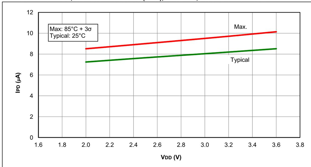
**FIGURE 30-39: I<sub>PD</sub>, BROWN-OUT RESET (BOR), BORV = 0, PIC16F1508/9 ONLY**
