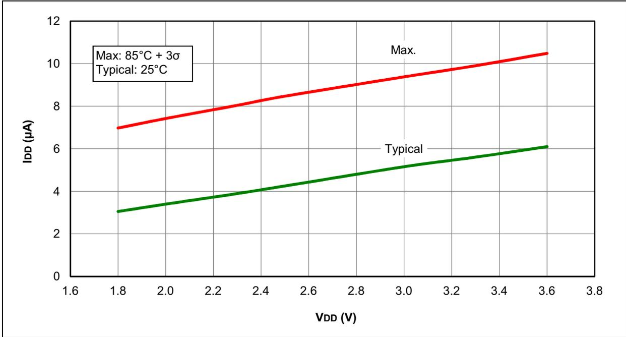
FIGURE 30-20:  $I_{DD}$ , LFINTOSC,  $F_{osc} = 31$  kHz, PIC16F1508/9 ONLY
