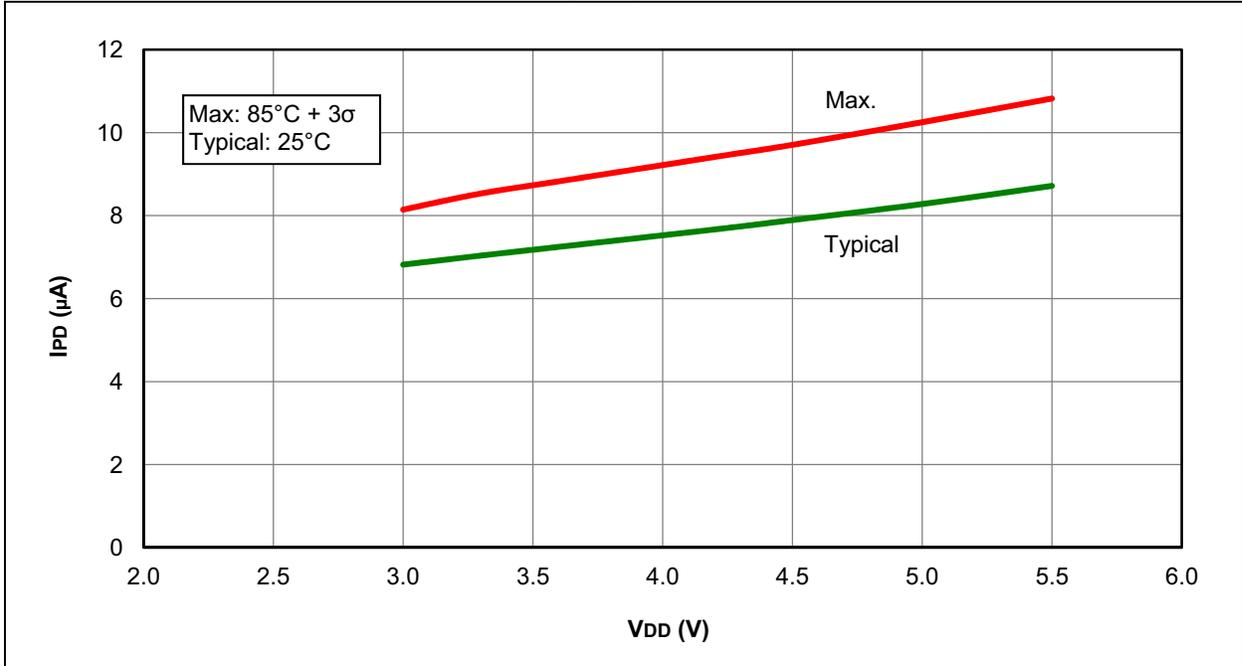
**FIGURE 30-40: I<sub>PD</sub>, BROWN-OUT RESET (BOR), BORV = 1, PIC16F1508/9 ONLY**
