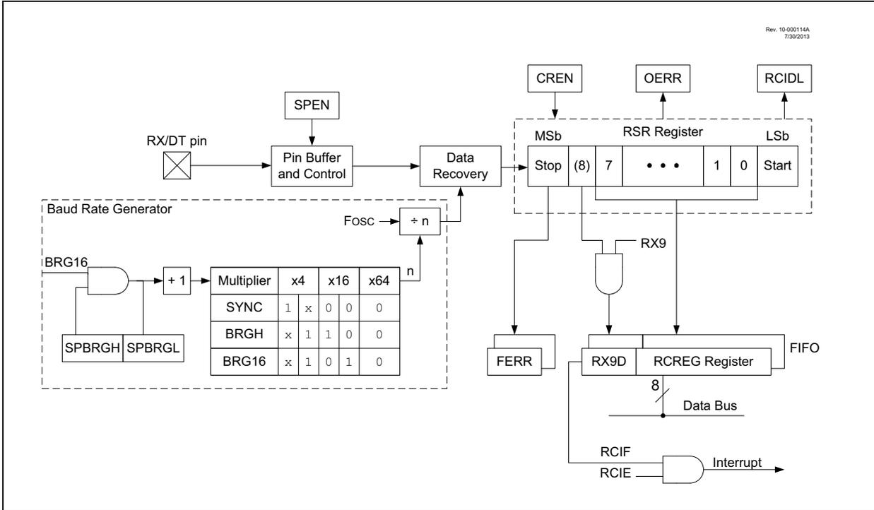
The operation of the EUSART module is controlled through three registers:
