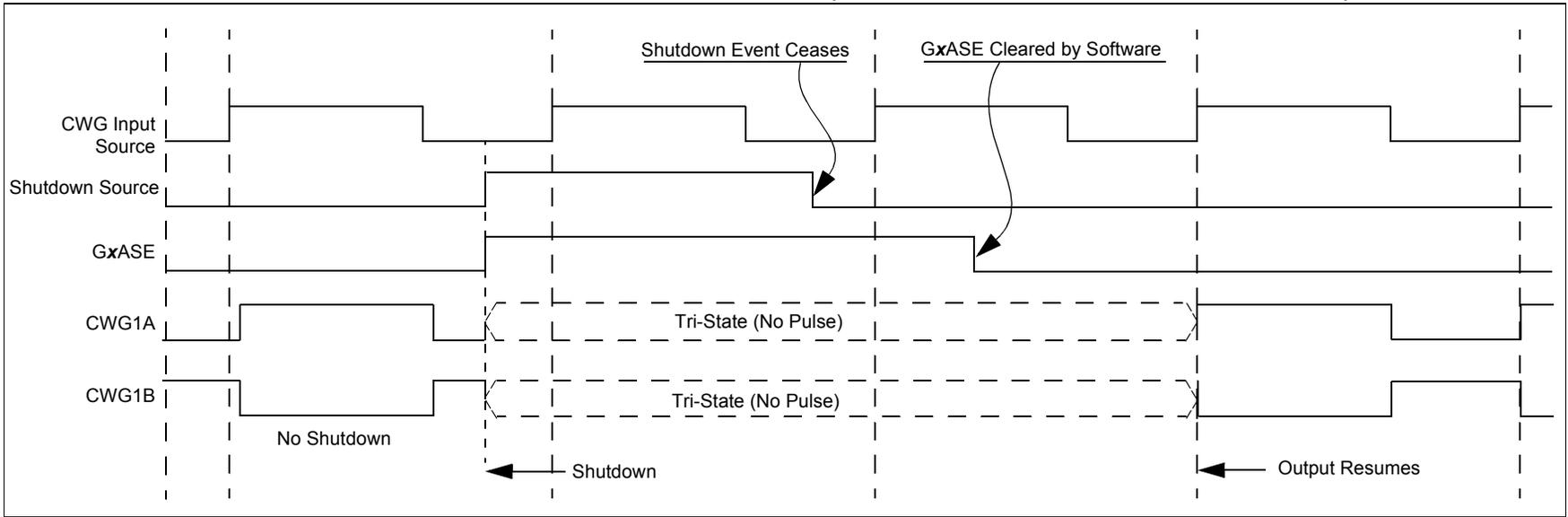
**FIGURE 26-6: SHUTDOWN FUNCTIONALITY, AUTO-RESTART ENABLED (GxARSEN = 1, GxASDLA = 01, GxASDLB = 01)**
