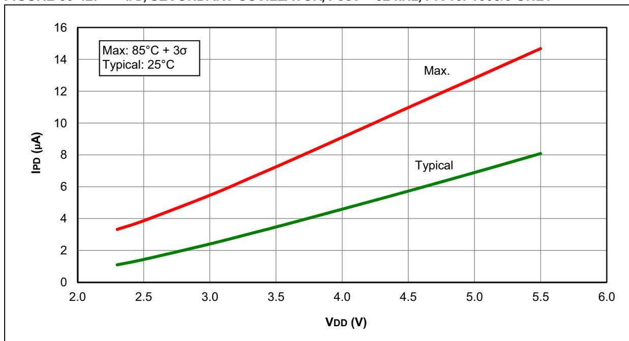
**FIGURE 30-43: I<sub>PD</sub>, COMPARATOR, LOW-POWER MODE (C<sub>x</sub>SP = 0), PIC16LF1508/9 ONLY**
