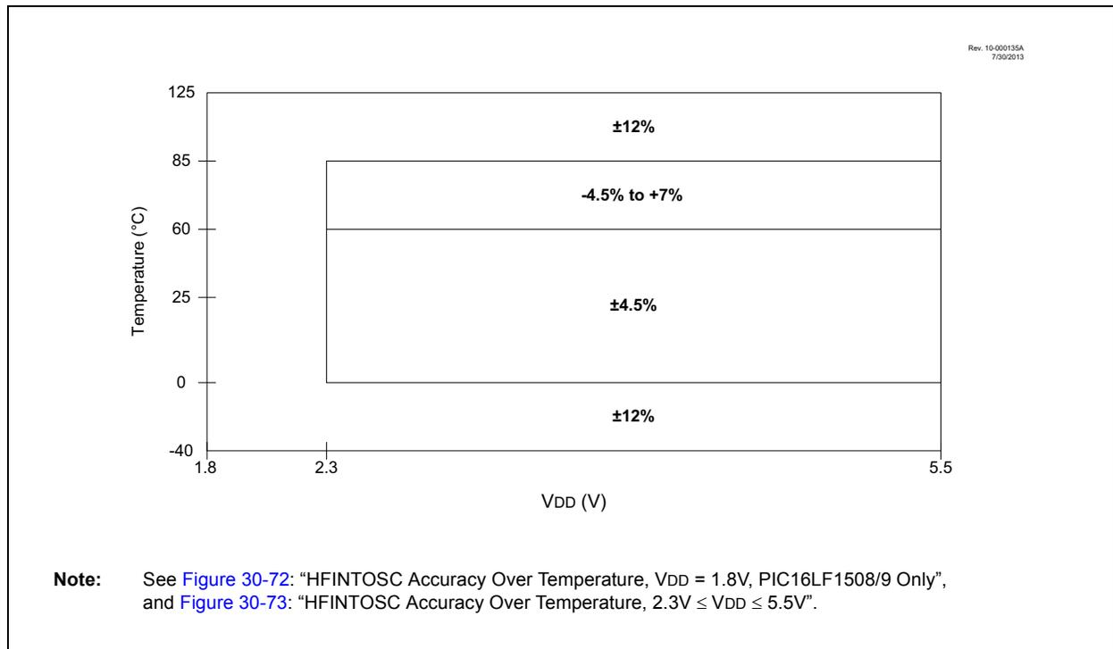
**Note:** See [Figure 30-72](#): "HFINTOSC Accuracy Over Temperature, V<sub>DD</sub> = 1.8V, PIC16LF1508/9 Only", and [Figure 30-73](#): "HFINTOSC Accuracy Over Temperature, 2.3V ≤ V<sub>DD</sub> ≤ 5.5V".
