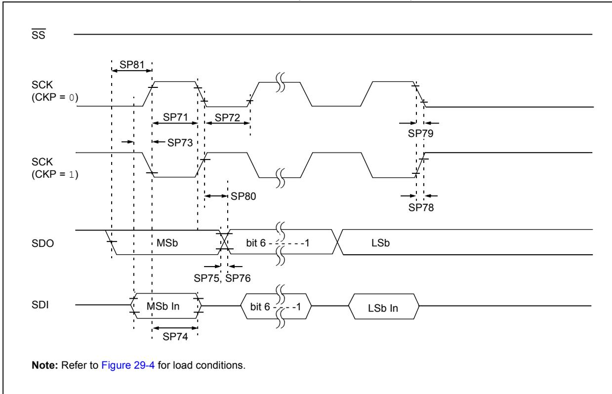
**FIGURE 29-18: SPI SLAVE MODE TIMING (CKE = 0)**
