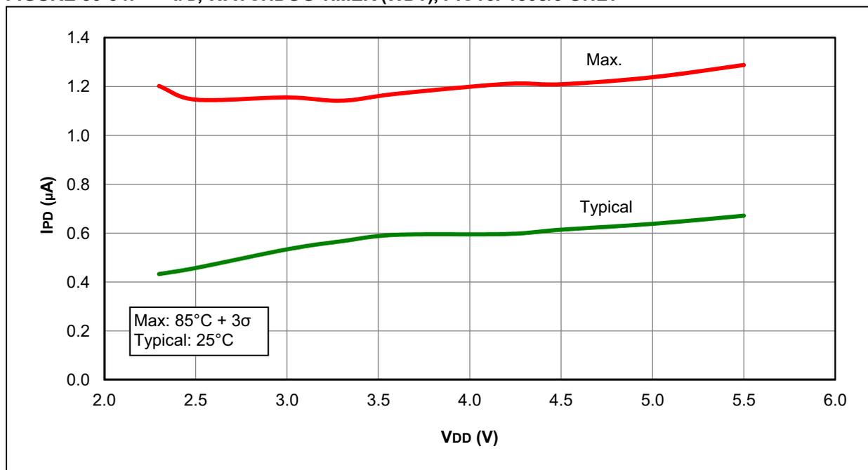
**FIGURE 30-35: I<sub>PD</sub>, FIXED VOLTAGE REFERENCE (FVR), PIC16LF1508/9 ONLY**
