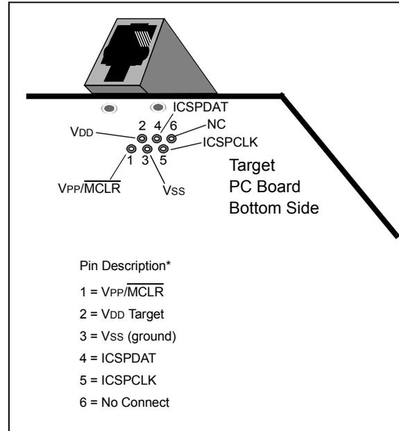
Another connector often found in use with the PICkit™ programmers is a standard 6-pin header with 0.1 inch spacing. Refer to [Figure 27-2](#).
