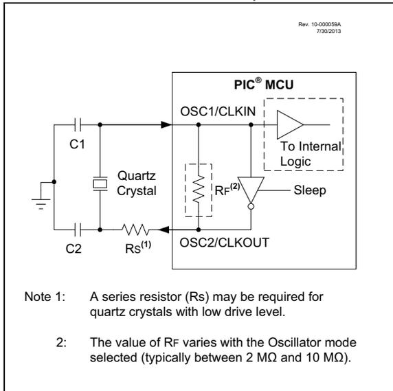
**Note 1:** Quartz crystal characteristics vary according to type, package and manufacturer. The user should consult the manufacturer data sheets for specifications and recommended application.
