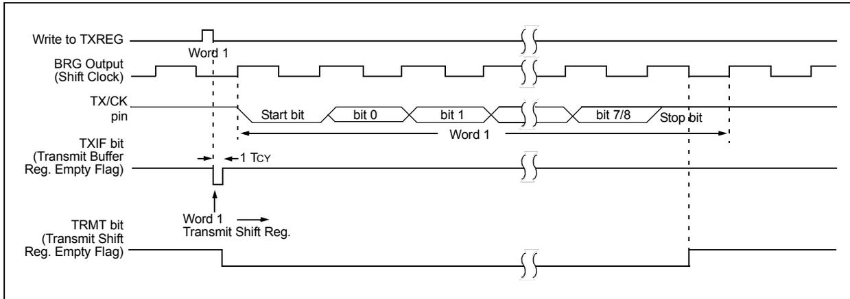
**FIGURE 22-4: ASYNCHRONOUS TRANSMISSION (BACK-TO-BACK)**
