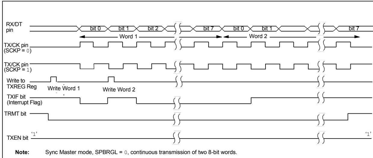
**FIGURE 22-11: SYNCHRONOUS TRANSMISSION (THROUGH TXEN)**
