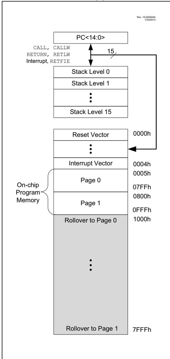
**FIGURE 3-2: PROGRAM MEMORY MAP AND STACK FOR PIC16(L)F1509**
