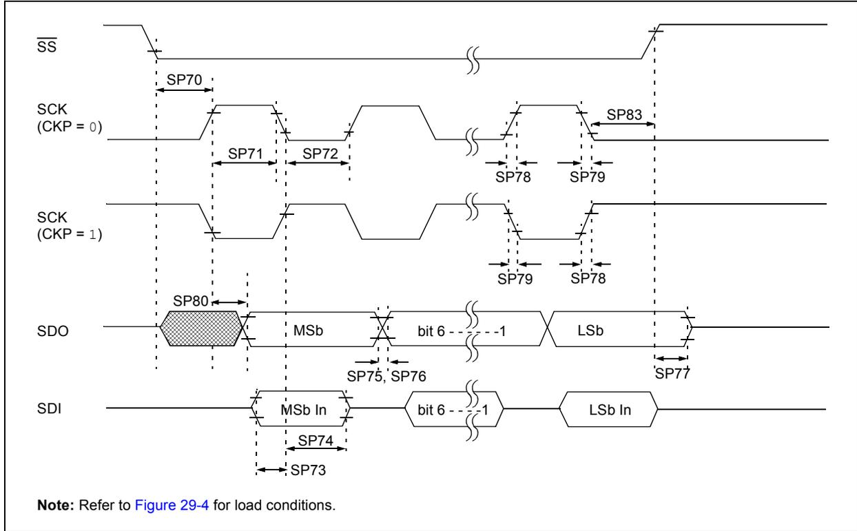
**FIGURE 29-19: SPI SLAVE MODE TIMING (CKE = 1)**
