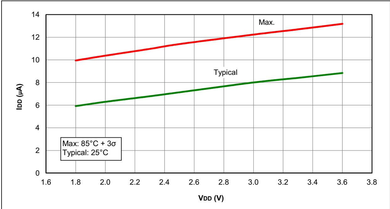
**FIGURE 30-8: I<sub>DD</sub>, EXTERNAL CLOCK (ECL), LOW-POWER MODE, F<sub>osc</sub> = 32 kHz, PIC16F1508/9 ONLY**
