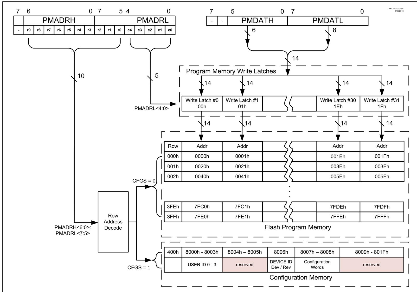
**FIGURE 10-6: FLASH PROGRAM MEMORY WRITE FLOWCHART**
