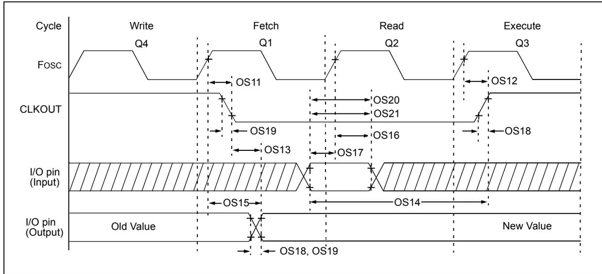
**TABLE 29-9: CLKOUT AND I/O TIMING PARAMETERS**
