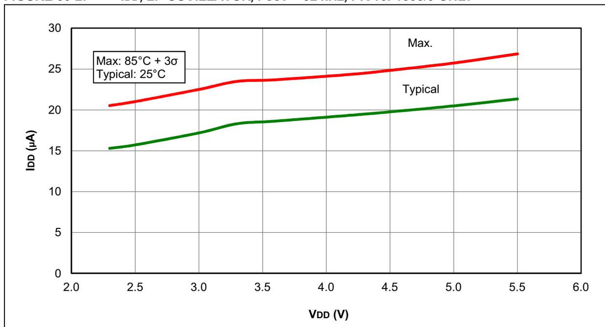
**FIGURE 30-3: I<sub>DD</sub> TYPICAL, XT AND EXTRC OSCILLATOR, PIC16LF1508/9 ONLY**
