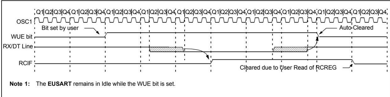
**FIGURE 22-8: AUTO-WAKE-UP BIT (WUE) TIMINGS DURING SLEEP**
