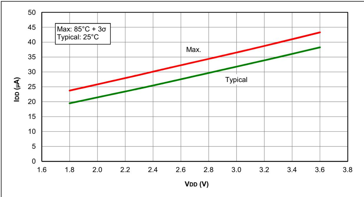
**FIGURE 30-10: I<sub>DD</sub>, EXTERNAL CLOCK (ECL), LOW-POWER MODE, F<sub>osc</sub> = 500 kHz, PIC16F1508/9 ONLY**
