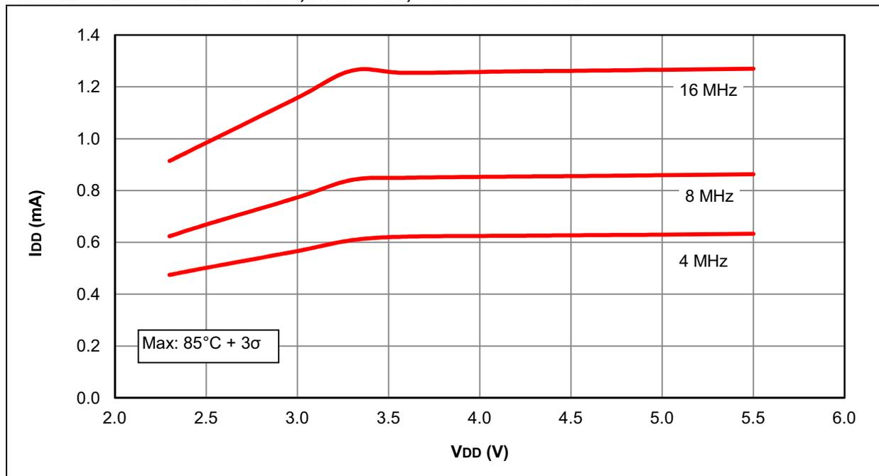
**FIGURE 30-27: I<sub>DD</sub> TYPICAL, HS OSCILLATOR, PIC16LF1508/9 ONLY**
