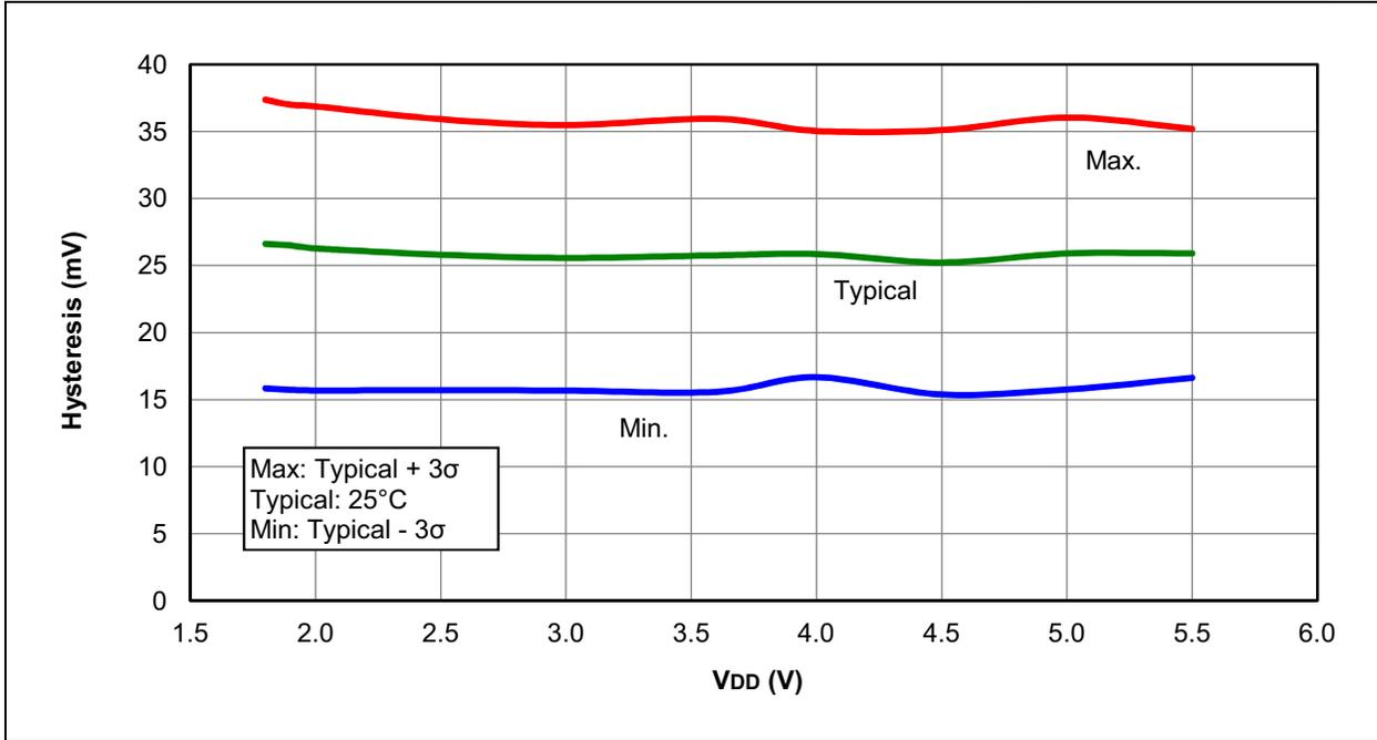
**FIGURE 30-66: COMPARATOR HYSTERESIS, LOW-POWER MODE (CxSP = 0, CxHYS = 1)**
