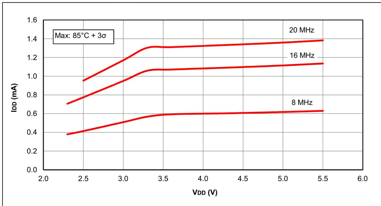
FIGURE 30-19:  $I_{DD}$ , LFINTOSC,  $F_{osc} = 31$  kHz, PIC16LF1508/9 ONLY
