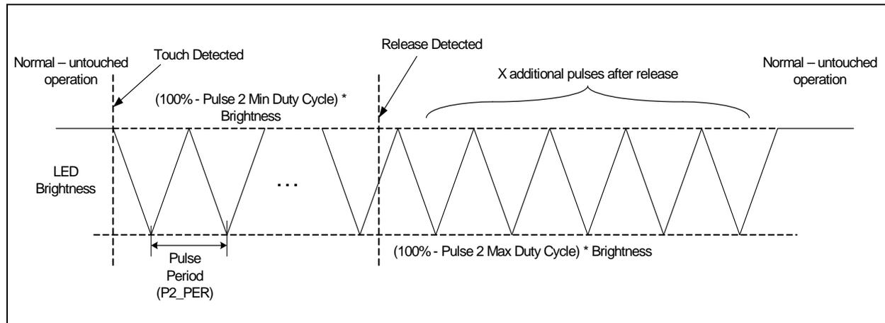
Figure 5.3 Pulse 2 Behavior with Non-Inverted Polarity
