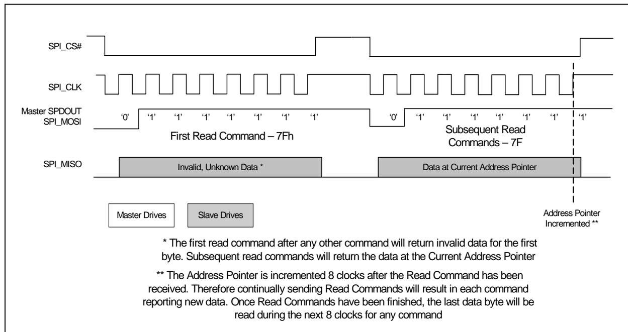
Figure 3.7 SPI Read Command - Normal Mode
