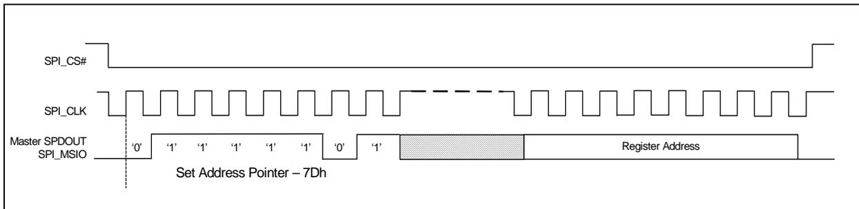
Figure 3.10 SPI Set Address Pointer Command - Bi-directional Mode
