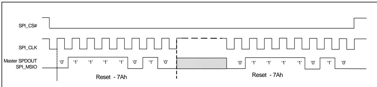
Figure 3.9 SPI Reset Interface Command - Bi-directional Mode
