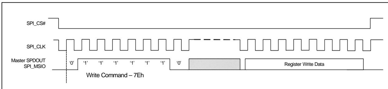
Figure 3.11 SPI Write Data Command - Bi-directional Mode
