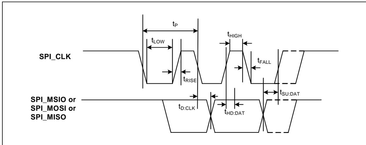
Figure 3.2 SPI Timing
