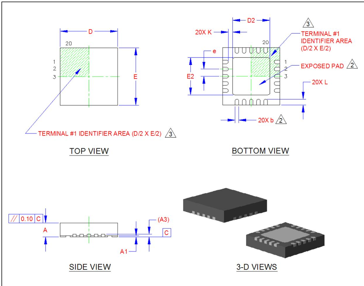
Figure 6.4 20-Pin QFN 4mm x 4mm Package Drawing
