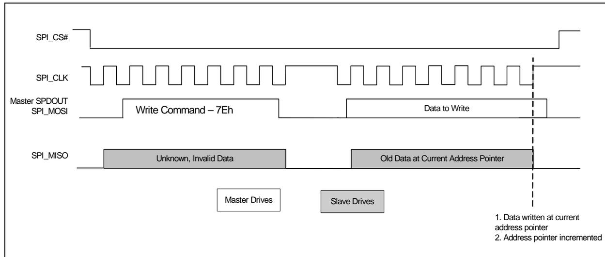
Figure 3.6 SPI Write Command - Normal Mode
