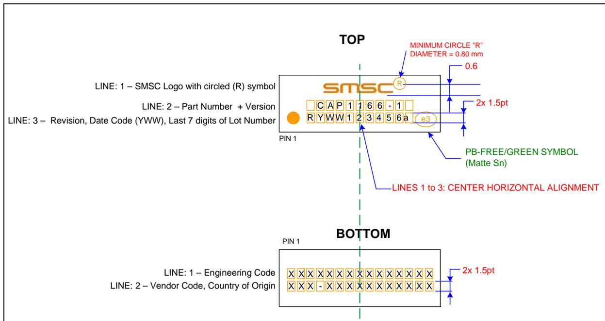
Figure 6.8 CAP1166 Package Markings - 24-Pin SSOP
