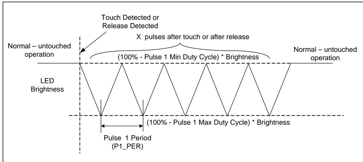
**Figure 5.1 Pulse 1 Behavior with Non-Inverted Polarity**
