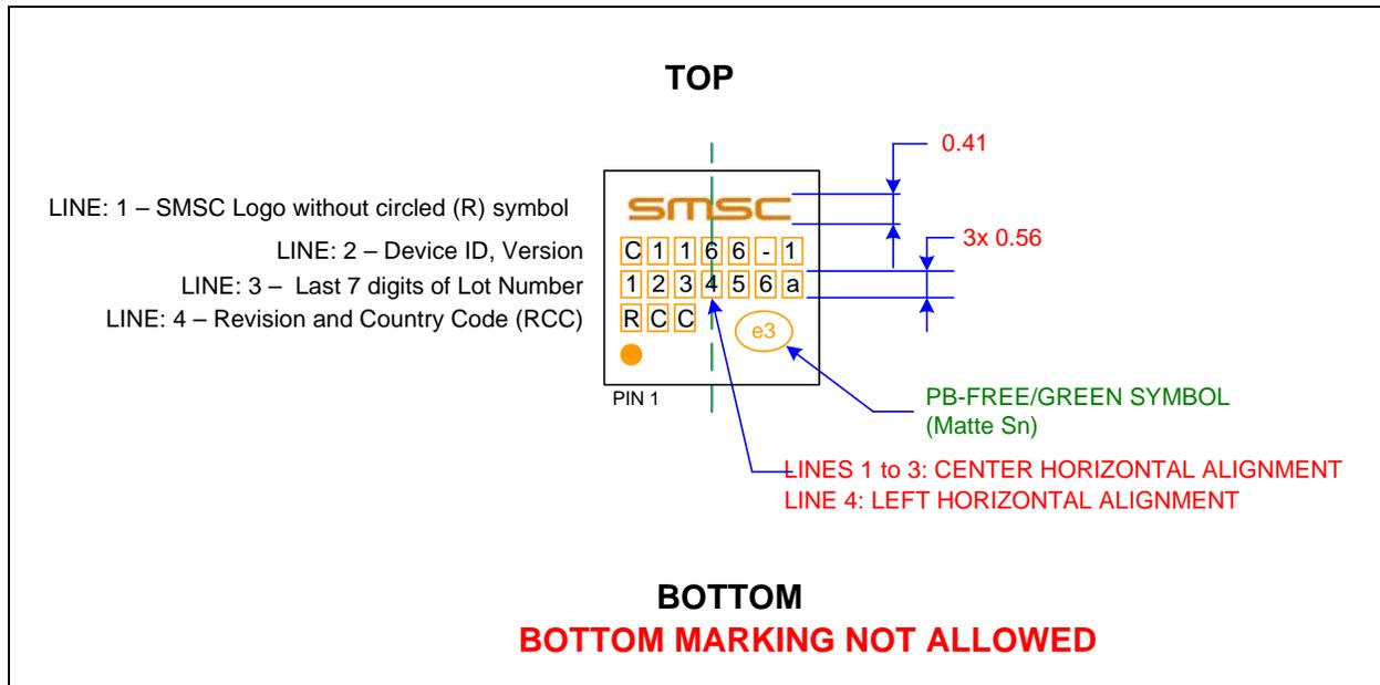
Figure 6.7 CAP1166 Package Markings - 20-Pin QFN
