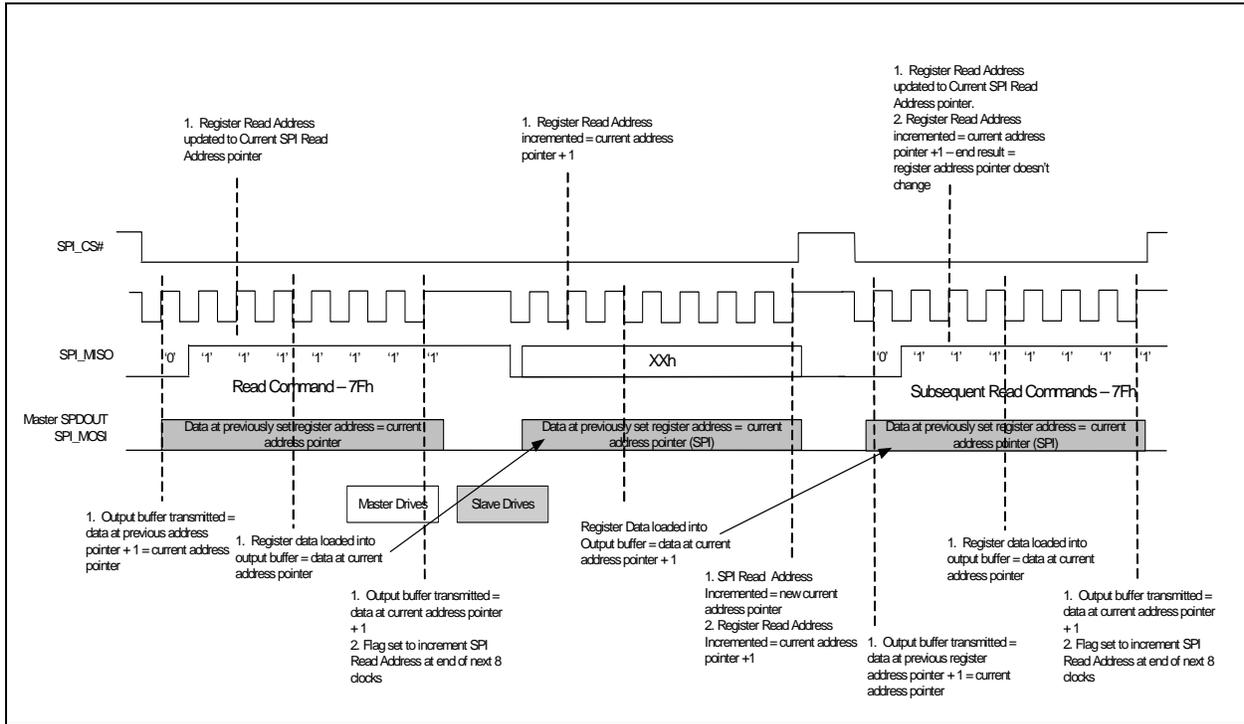
Figure 3.8 SPI Read Command - Normal Mode - Full
