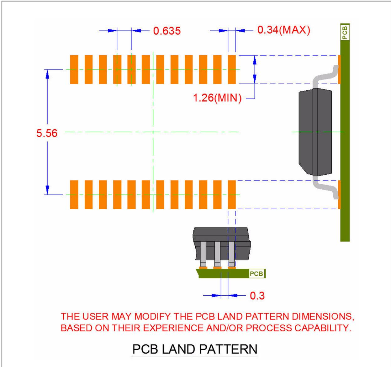
Figure 6.3 CAP1166 PCB Land Pattern - 24-Pin SSOP
