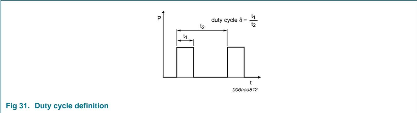
Fig 31. Duty cycle definition
