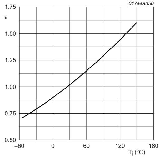
$$a = \frac{R_{DSon}}{R_{DSon(25^\circ C)}}$$
