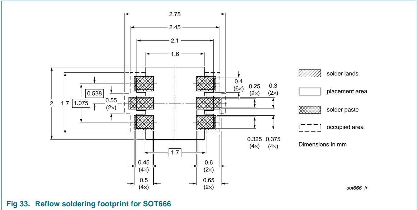
**Fig 33. Reflow soldering footprint for SOT666**
