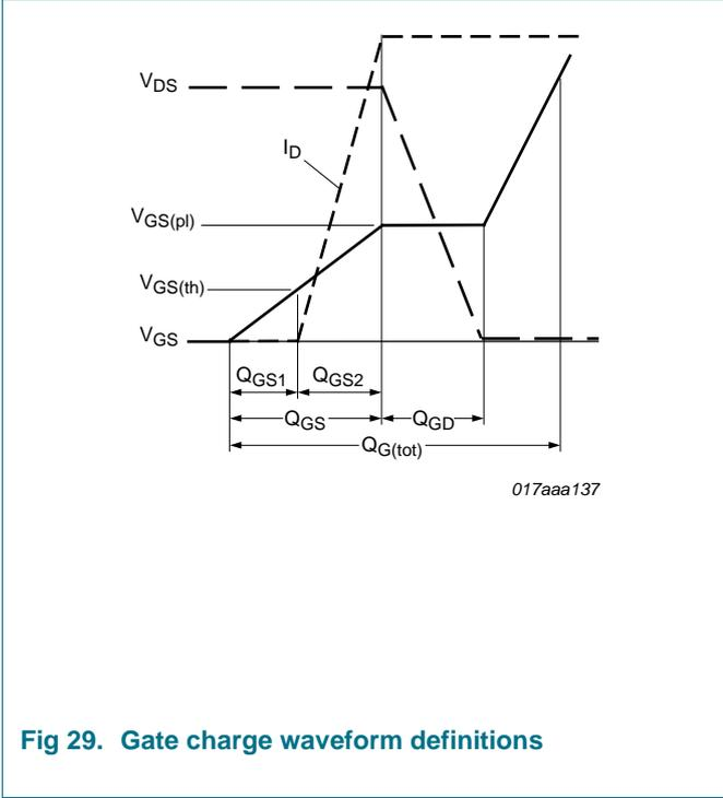
Fig 29. Gate charge waveform definitions
