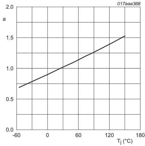
$$a = \frac{R_{DS(on)}}{R_{DS(on)(25^\circ\text{C})}}$$
