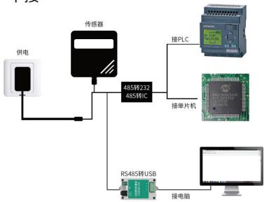
This product can also combine multiple sensors in one485Bus usage, theoretically a bus can254indivual485The other end of the sensor is connected to485InterfacePLC, pass485Interface chip connected to the microcontroller, or useUSBchange485It can be connected to the computer and use the sensor configuration tool provided by our company to configure and test (only one device can be connected when using this configuration software).
