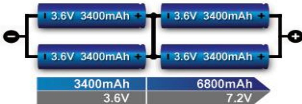
**Figure 6: Series/ parallel connection of four cells (2s2p).**
