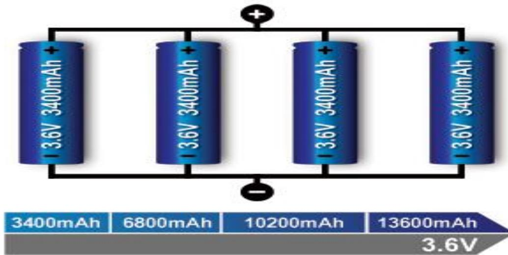
**Figure 4: Parallel connection of four cells (4p).**
