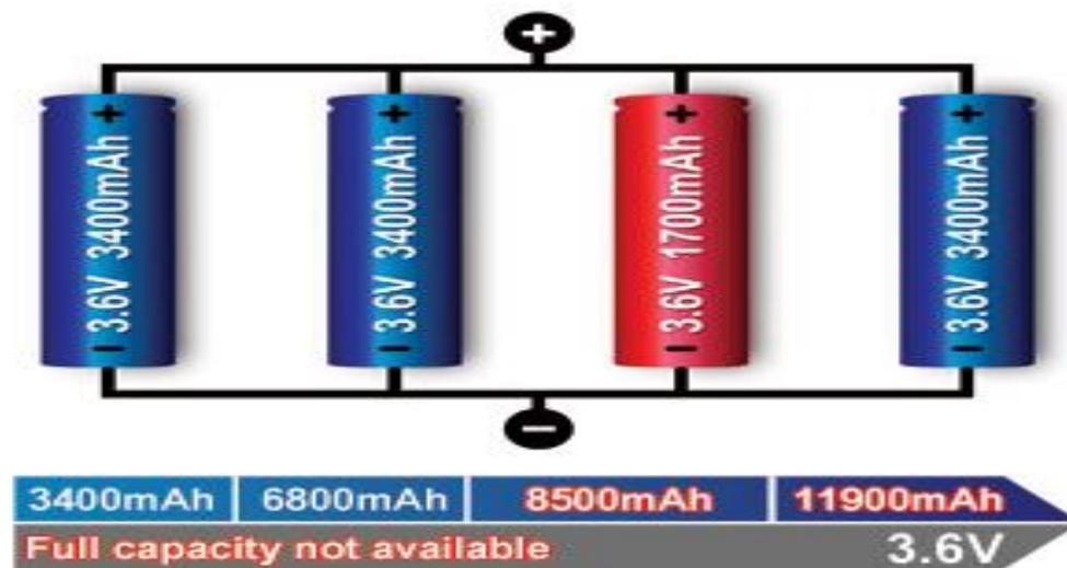
Figure 5: Parallel/connection with one faulty cell.
