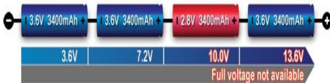
**Figure 3: Series connection with a faulty cell.**
