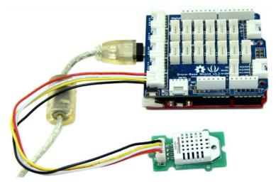
2. Download <u>Seeed DHT library</u> for arduino boards with 16MHz XTAL; Unzip and put it in the libraries file of Arduino IDE by the path: ..\arduino-1.0\libraries; Another library - <u>DHTlib</u> is also available instead of Seeed DHT library. This library supports both 16MHz and 8MHz Arduino (eg. Seeeduino Stalker)
