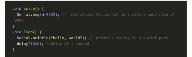
In the upper left corner of the Arduino IDE, there are two buttons, Verify and Upload. First, press the Verify button(✓) to compile. After the compilation is successful, press the upload button(→).
