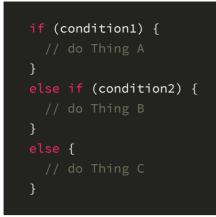
The usage of the statement is: if the logical expression in parentheses is true, execute the statement in curly braces after **if**, if not, execute the statement in curly braces after the **else**. If the state of the button is high, the LED pin outputs a high level and turn the LED on, else turn LED off.
