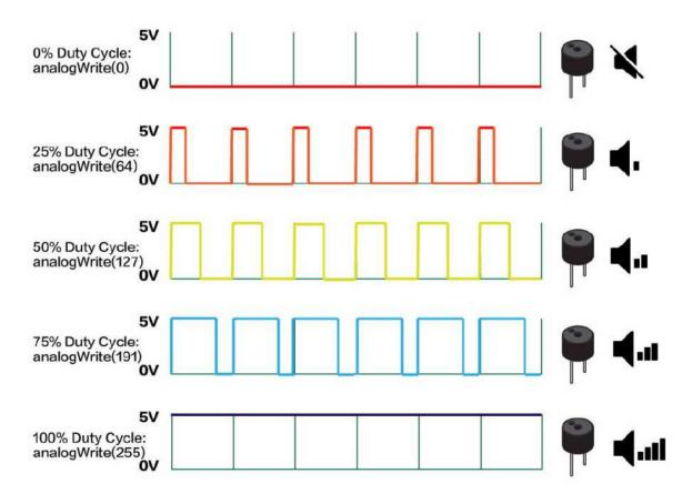
There are six digital pins on your Seeeduino that are marked with the symbol "~", which means they can send out a PWM signal : 3,5,6,9,10,11. They are celled PWM pins.
