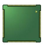
SIM7600EI is a complete multi-band LTE-FDD/LTE-TDD/HSPA+/UMTS/EDGE/GPRS/GSM module solution in LCC type which supports LTE CAT1 up to 10Mbps for downlink and 5Mbps for uplink data transfer. Designed in the compact and unified form factor, SIM7600EI is compatible with SIMCom HSPA+ SIM5360 module/LTE CAT3 SIM7100 and LTE CAT4 SIM7600E-H module, which allows customer to design their application once for different technology and benefit from great development time-saving.
