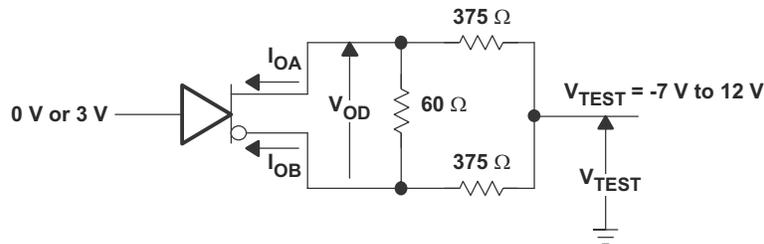
Figure 7-2. Driver Test Circuit,  $V_{OD}$  With Common-Mode Loading
