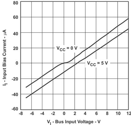
Figure 6-1. Bus Input Current versus Bus Input Voltage
