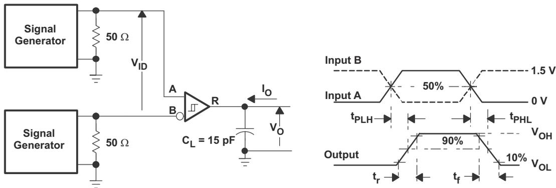
Figure 7-9. Receiver Switching Test Circuit and Waveforms
