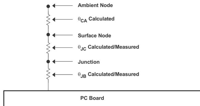
**Figure 11-2. Thermal Resistance**
