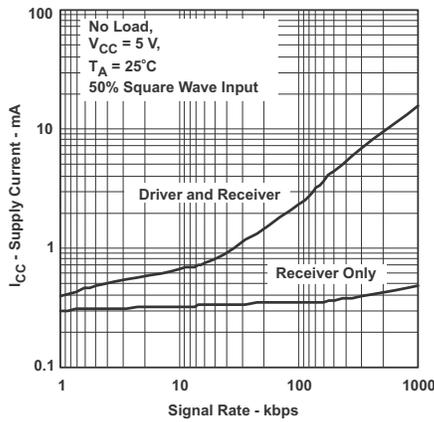
Figure 6-3. SN65HVD3085E RMS Supply Current versus Signaling Rate
