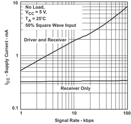
Figure 6-2. SN65HVD3082E RMS Supply Current versus Signaling Rate
