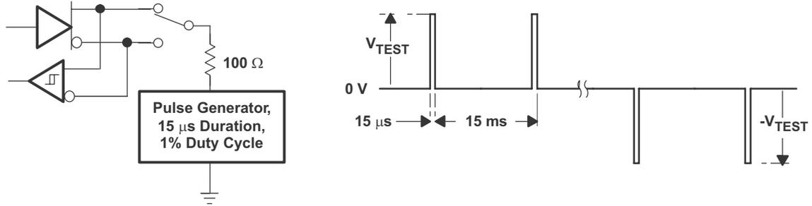
Figure 7-13. Test Circuit and Waveforms, Transient Overvoltage Test
