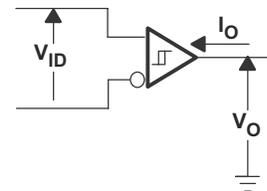
Figure 7-8. Receiver Switching Test Circuit and Waveforms
