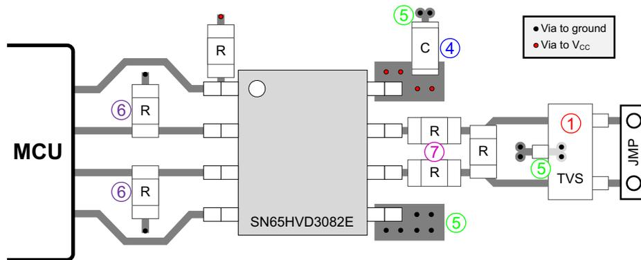
Figure 11-1. SNx5HVD308xE Layout Example
