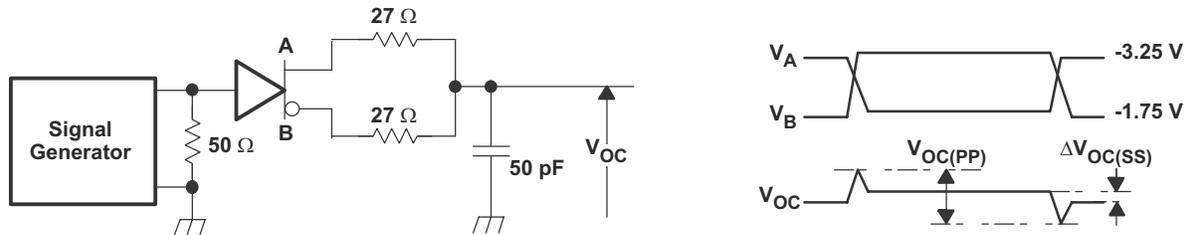
Figure 7-3. Driver  $V_{OC}$  Test Circuit and Waveforms
