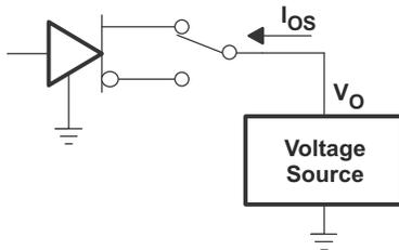
Figure 7-7. Driver Short-Circuit
