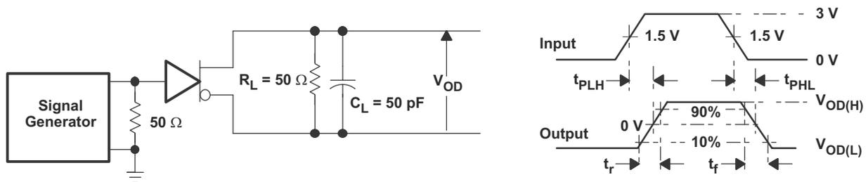
Figure 7-4. Driver Switching Test Circuit and Waveforms
