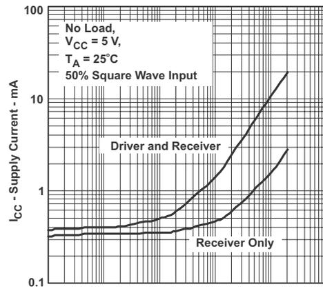
Figure 6-4. SN65HVD3088E RMS Supply Current versus Signal Rate
