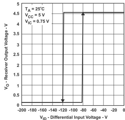
Figure 6-6. Receiver Output Voltage versus Differential Input Voltage
