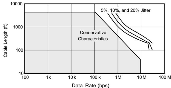
**Figure 9-3. Cable Length vs Data Rate Characteristic**
