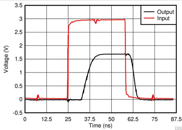
Figure 6-3. Switching Characteristics at 15 MHz Excellent Signal Integrity
