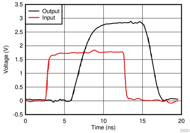
Figure 6-1. Switching Characteristics at 50 MHz Excellent Signal Integrity
