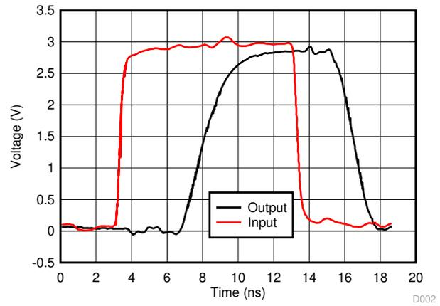
Figure 6-2. Switching Characteristics at 50 MHz Excellent Signal Integrity
