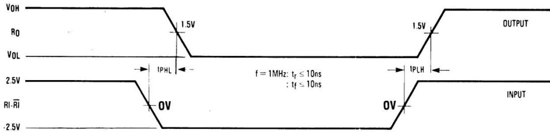
Note: Differential input voltage may be realized by grounding RI and pulsing RI between +2.5V and -2.5V
