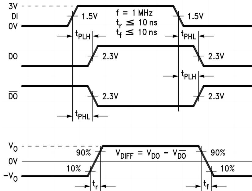
Figure 6. Driver Propagation Delays and Transition Times
