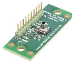
MPR Series with short port mounted on a breakout board.
