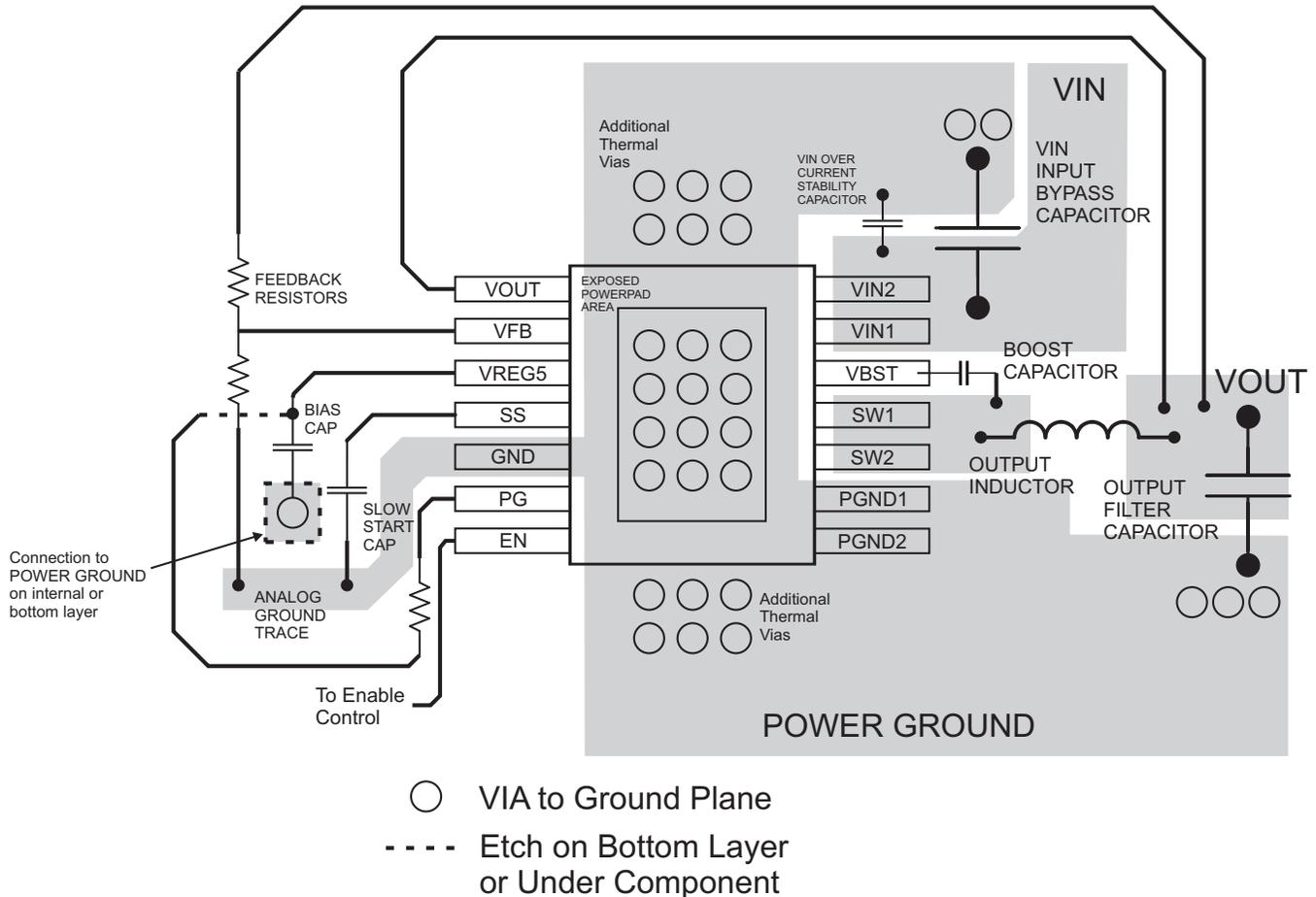
Figure 15. PCB Layout
