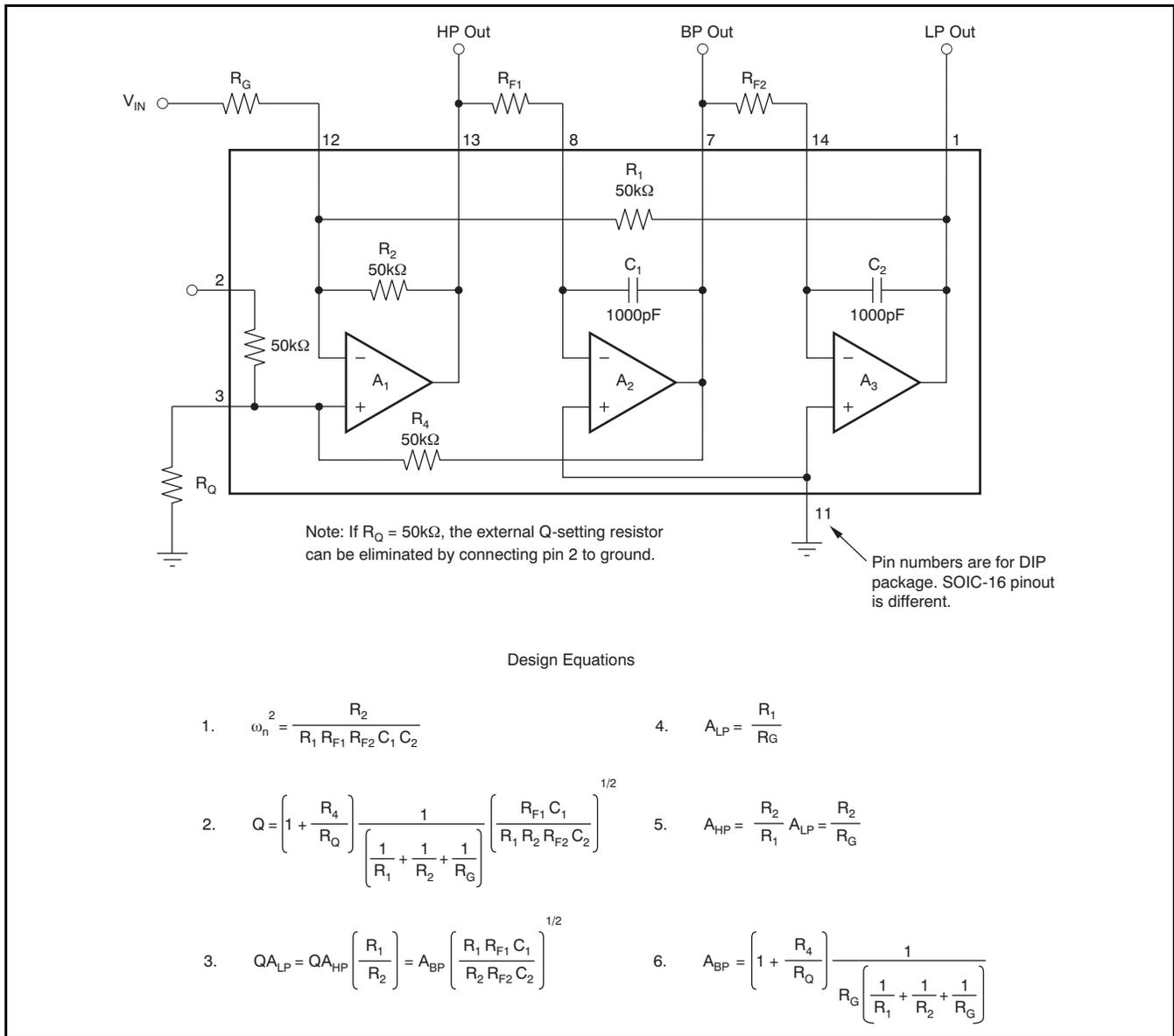
Figure 2. Inverting Pole-Pair
