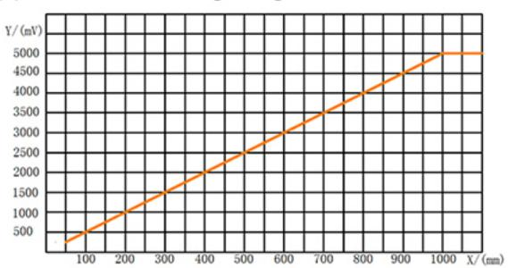
Note: The X-axis represents distance, and the Y-axis represents voltage.
