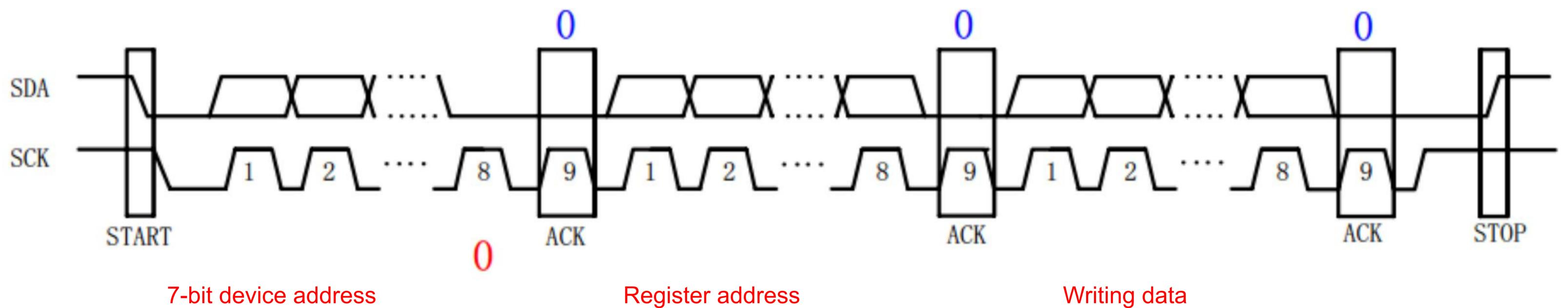
Note :When the communication rate exceeds 40 k bit/s, a 20us delay is increased after the descending edge of the ninth SCK clock (after the ACK position)
