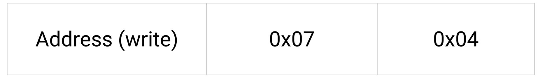
The module was modified from the detection angle level to level 4.
