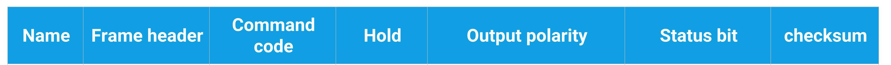
Note : checksum = (frame header + command code + output polarity + status bit)&0x00FF
