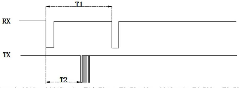
Remark: A01A and A01B series: T1 >70ms, T2=50~60ms A01C series T1≥500ms,T2≈500ms
