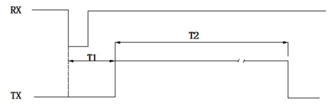
Remark: T1=1~8ms; T2=1.4~45ms (Timing of PWM High-level pulse width)
