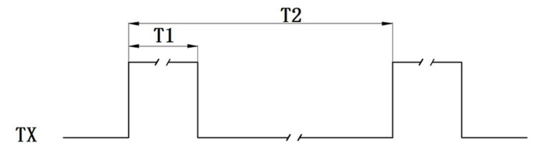
Remark: A01A and A01B series module Auto output: T1=1.4~45ms; T2=250ms
