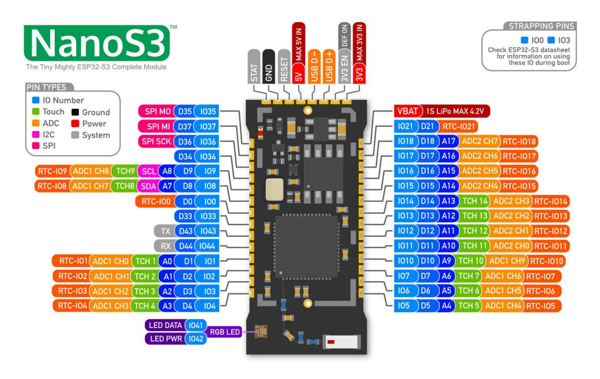
**Board Dimensions** 28mm x 11mm **Max Thickness** 2.4mm
