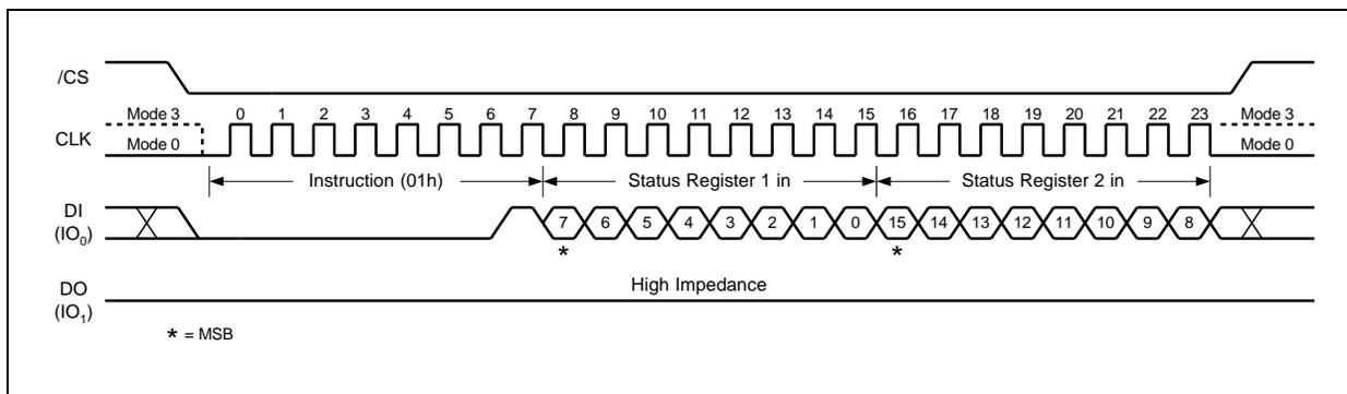
Figure 8. Write Status Register Instruction Sequence Diagram
