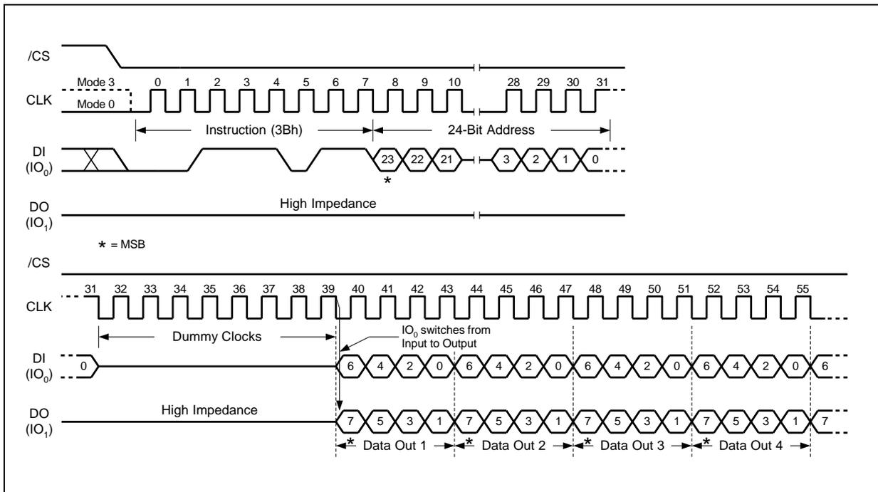
Figure 11. Fast Read Dual Output Instruction Sequence Diagram
