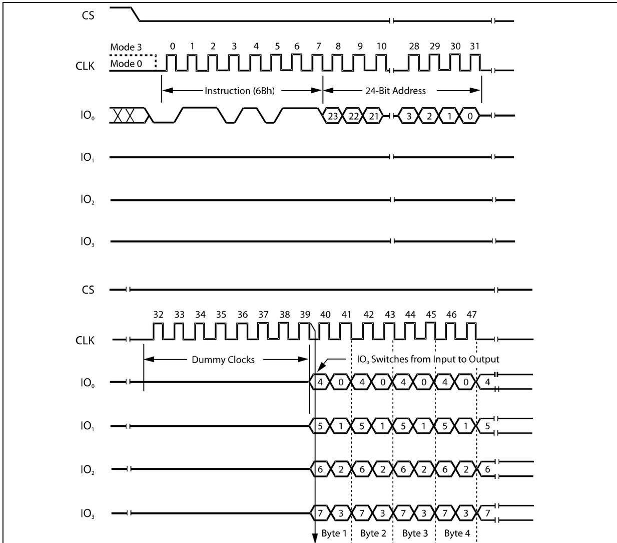
Figure 12. Fast Read Quad Output Instruction Sequence Diagram
