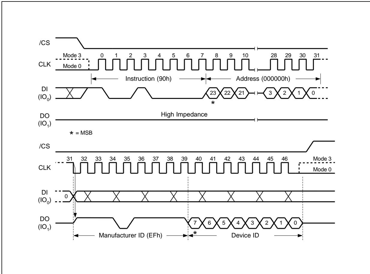
Figure 29. Read Manufacturer / Device ID Diagram
