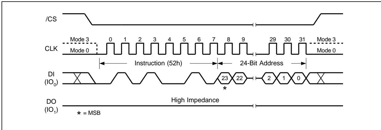
Figure 22a. 32KB Block Erase Instruction Sequence Diagram
