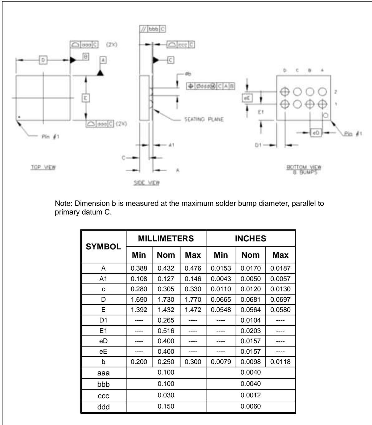
Note: Dimension b is measured at the maximum solder bump diameter, parallel to primary datum C.
