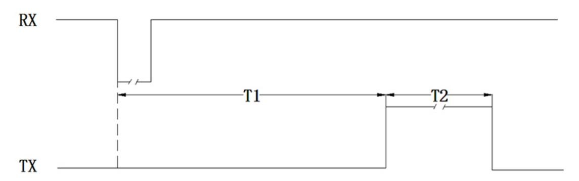
Remark: T1=0.9s~2.5s; T2=1.4ms~50ms (Timing of PWM High-level pulse width)
