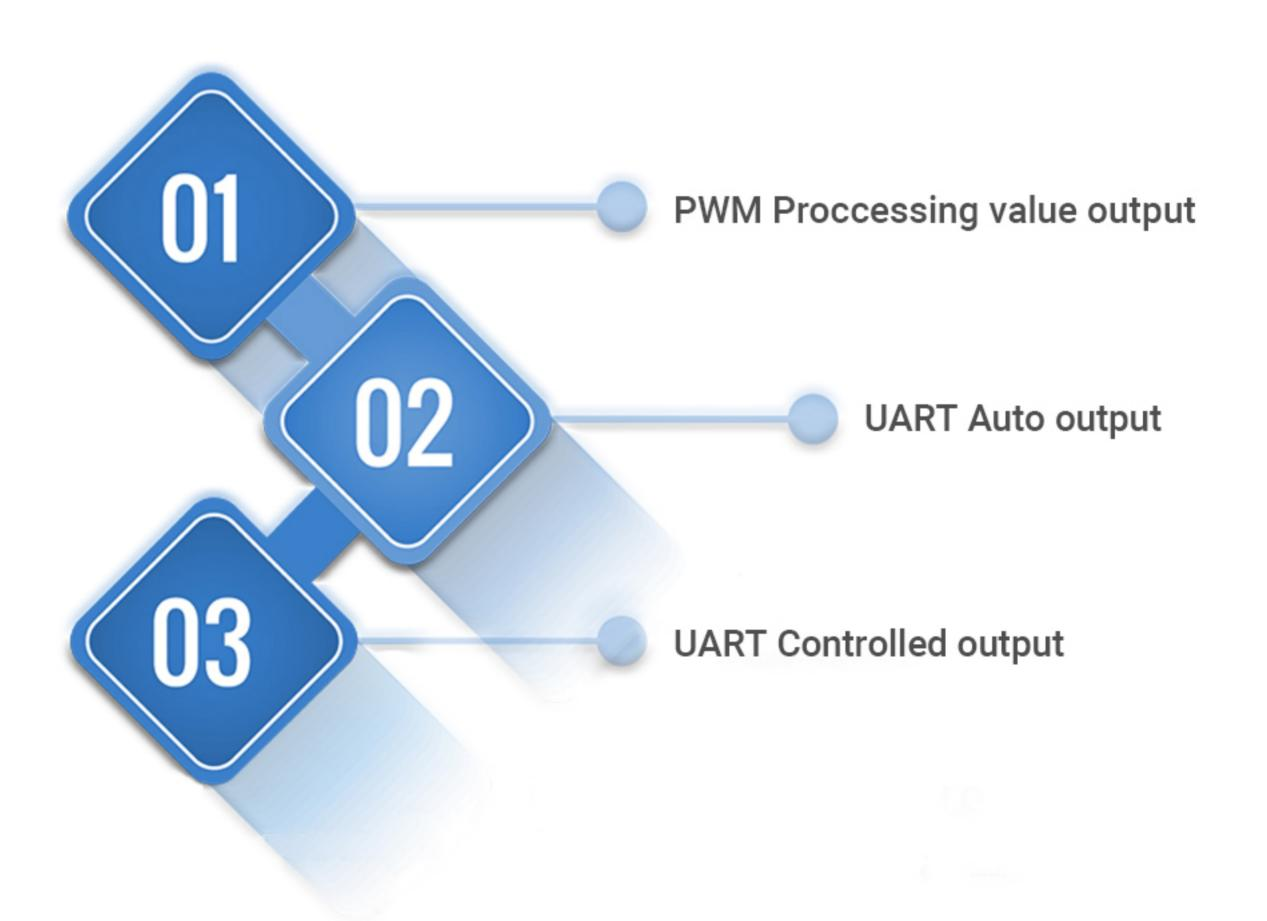
The module has three output modes including PWM processing value output, UART auto output, UART controlled output which set by software. Choose different models to set the module to different output modes.
