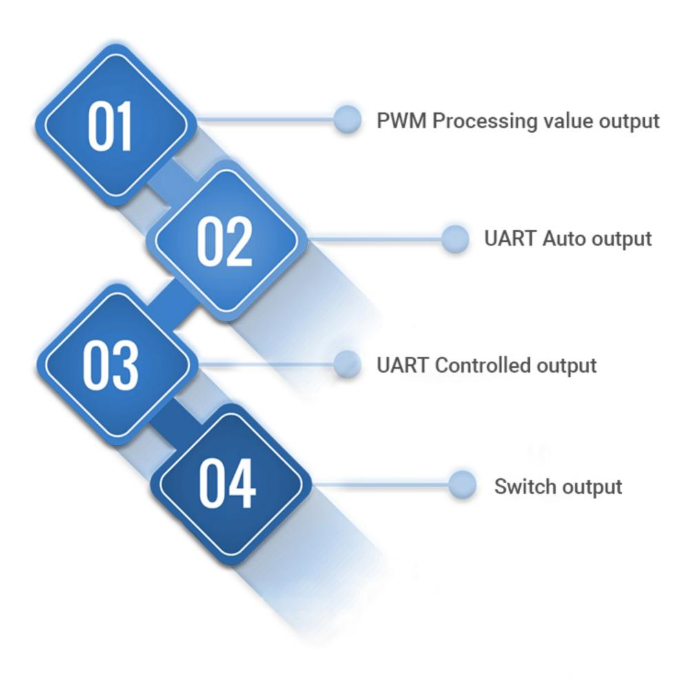
The module has four output modes: PWM processing value output, UART automatic output, UART controlled output and switch output, which are mainly set by software. Choose different models to set the module to different output modes.
