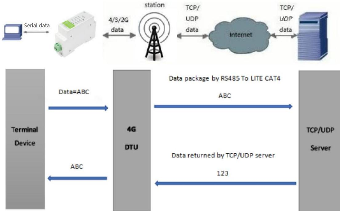
Figure Network Transparent Transmission
