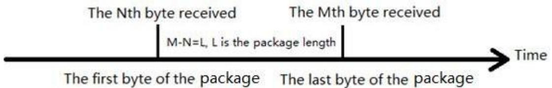
Figure Length Trigger
