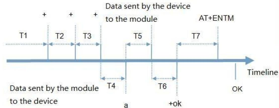
Figure Switching Command Mode Timing
