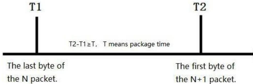
Figure Time Trigger Mode
