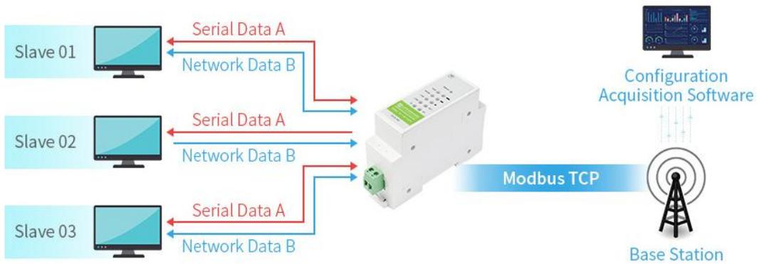
Figure Schematic diagram of ModbusTCP/RTU protocol mutual conversion function
