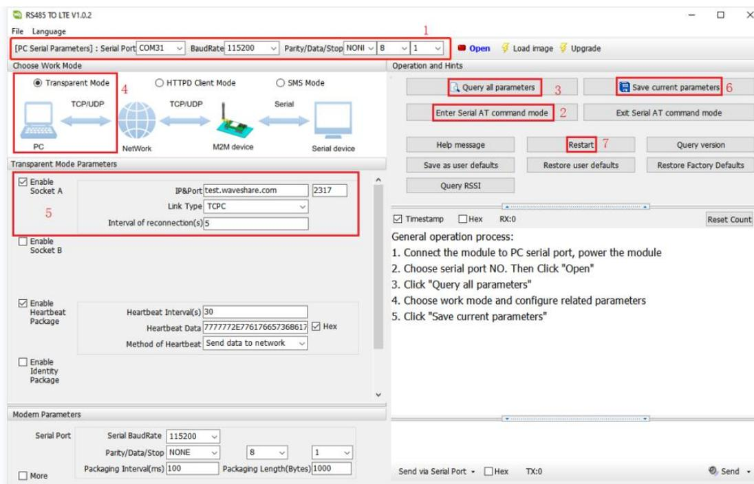
Figure Software Setup
