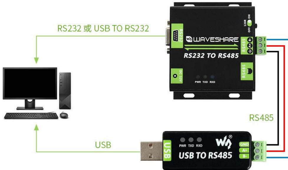
Open two SSCOM software on host PC. Select the correct serial port and set their baud rate to the same, check the SendEvery option. Then you can test if the devices can transmit and receive normally.
