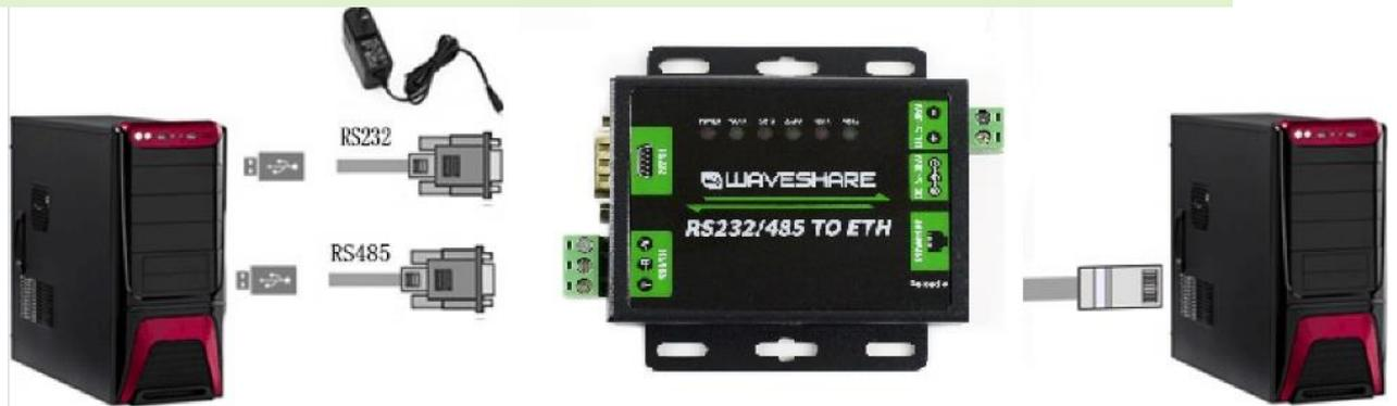
Figure 1 Application Diagram
