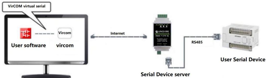
Figure 12 Application example of virtual serial port
