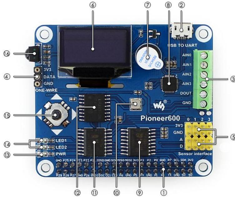
1. Raspberry Pi GPIO interface: for connecting Raspberry Pi
